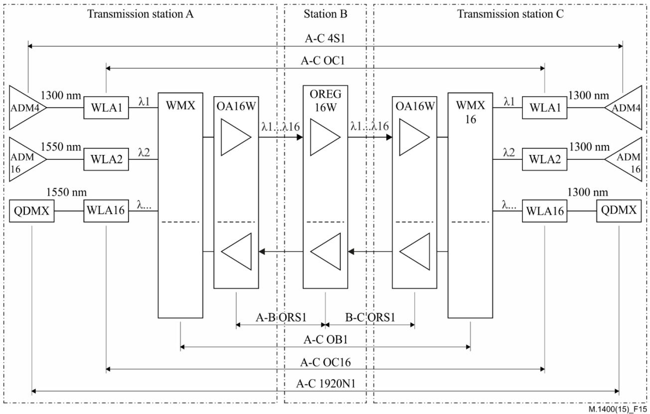
**Figure 15 – Example of the DWDM scheme with the function codes**
