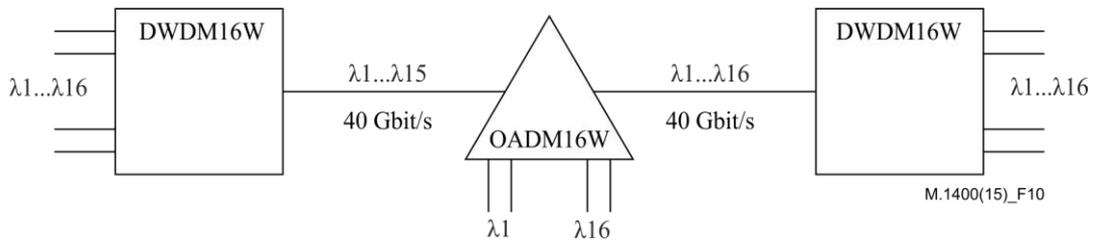
**Figure 10 – Example of an optical add-drop multiplexer 16 wavelengths with 2 wavelengths extracted and inserted**
