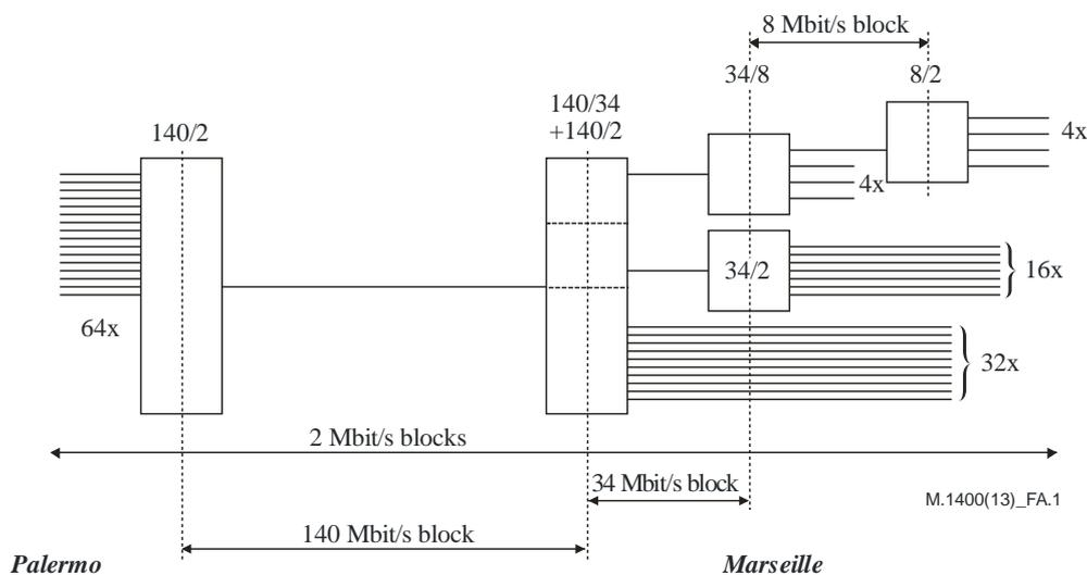
**Figure A.1 – Digital block bidirectional asymmetrical configuration**
