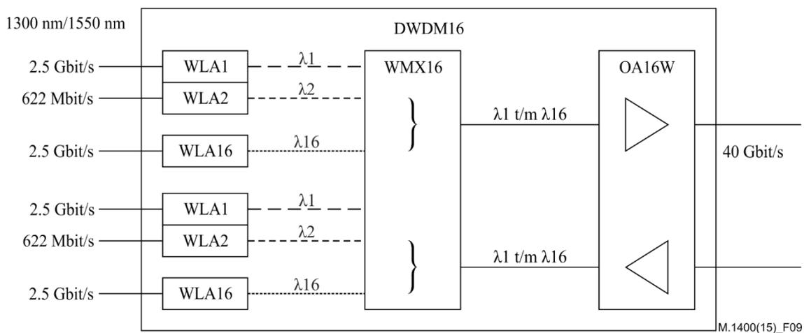
**Figure 9 – Example of the equipment on one side with 16 wavelengths**
