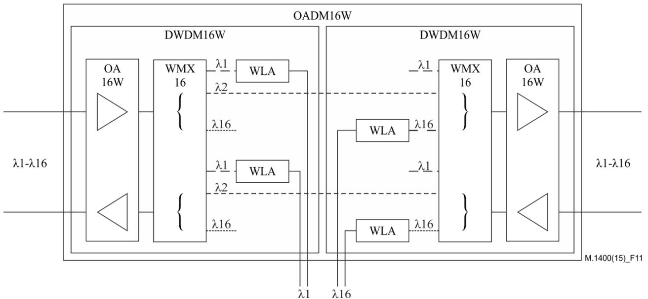
**Figure 11 – Detail of the optical add-drop multiplexer 16 wavelengths with 2 wavelengths extracted and inserted**
