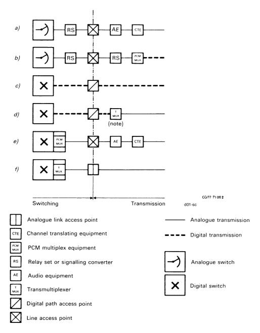
Note - The transmultiplexer shown could also be a PCM multiplex equipment/channel translating equipment combination.
