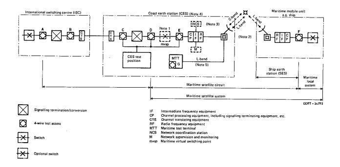
Note 1 — A maritime virtual switching point should always be established for transmission planning purposes. However, a switch at the coast earth station is optional.
