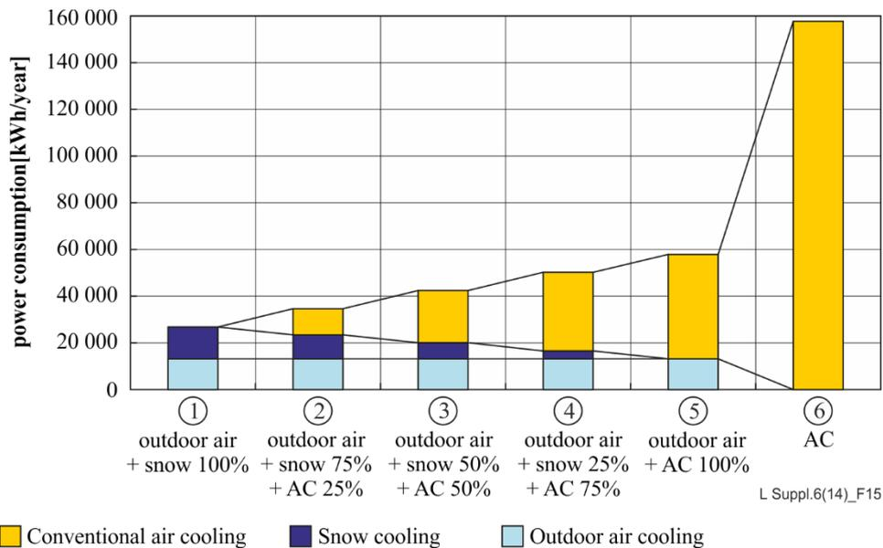
**Figure 15 – Calculated annual power consumption of the test facility**
