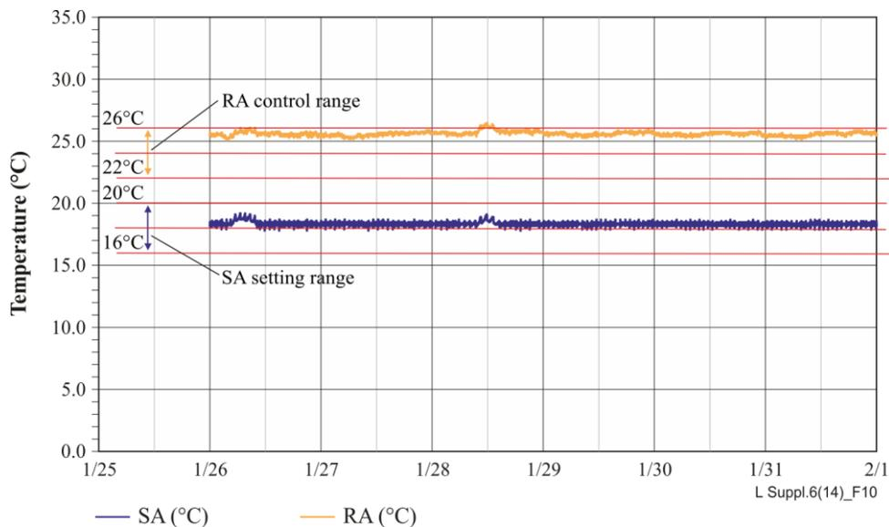
**Figure 10 – Air temperature in snow and ice cooling**
