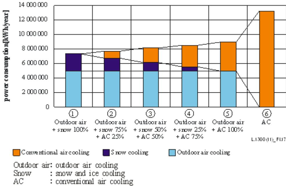
**Figure 17 – Calculated annual power consumption of the 1000-rack model data centre**
