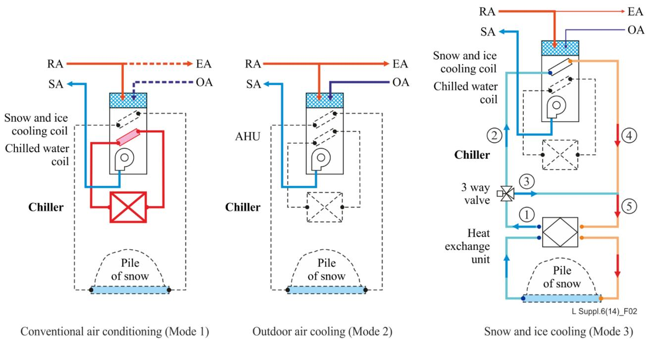
**Figure 2 – Image of each cooling mode**
