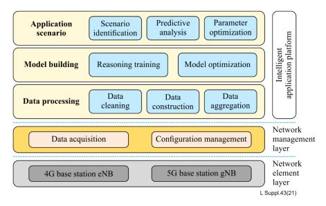
Figure 2 – Overall architecture of a 5G intelligent energy-saving network
