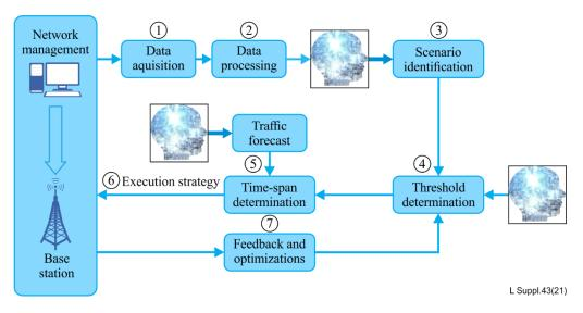
Figure 3 – AI energy-saving procedure for a 5G base station
