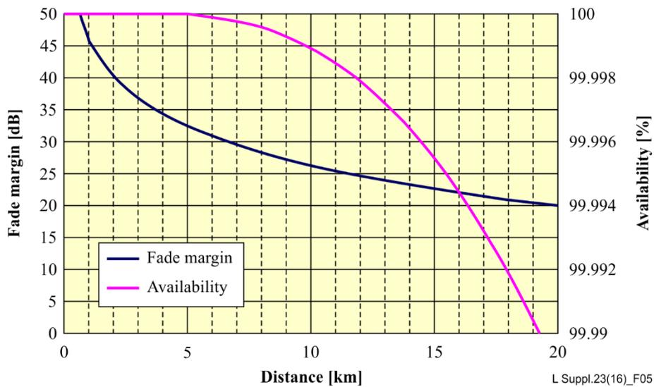
**Figure 5 – Example of link budget calculation at 13 GHz:
