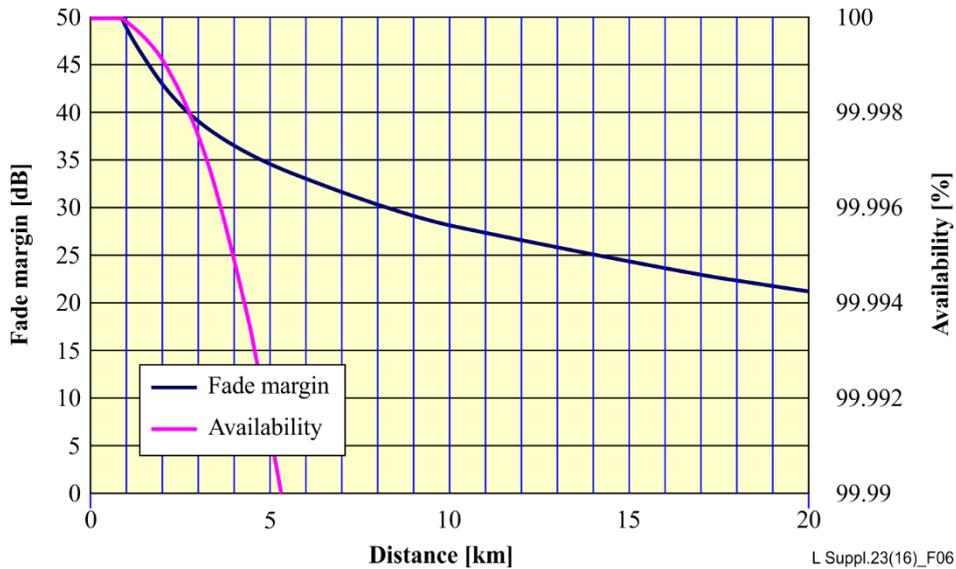
**Figure 6 – Example of link budget calculation at 38 GHz:
