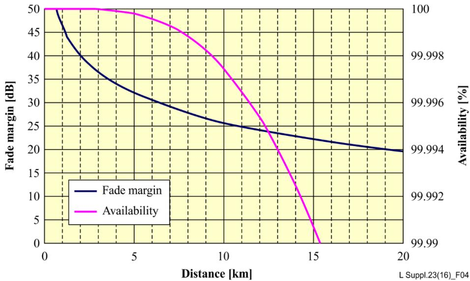
**Figure 4 – Example of link budget calculation at 15 GHz:
