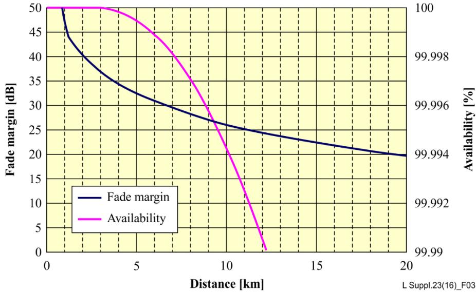
**Figure 3 – Example of link budget calculation at 18 GHz:
