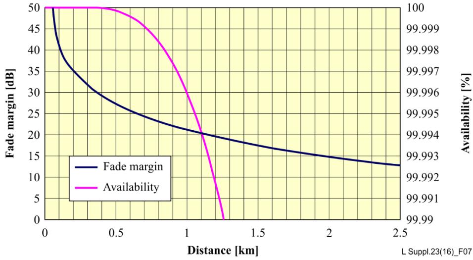
**Figure 7 – Example of link budget calculation at 80 GHz:
