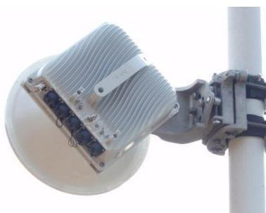
**Figure II.1 – Example of E-band (71-76 GHz, 81-86 GHz) wireless link**
