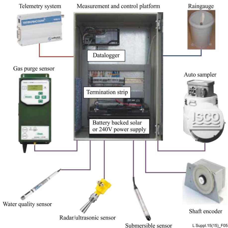
Figure 5 – Typical water quality station equipment
