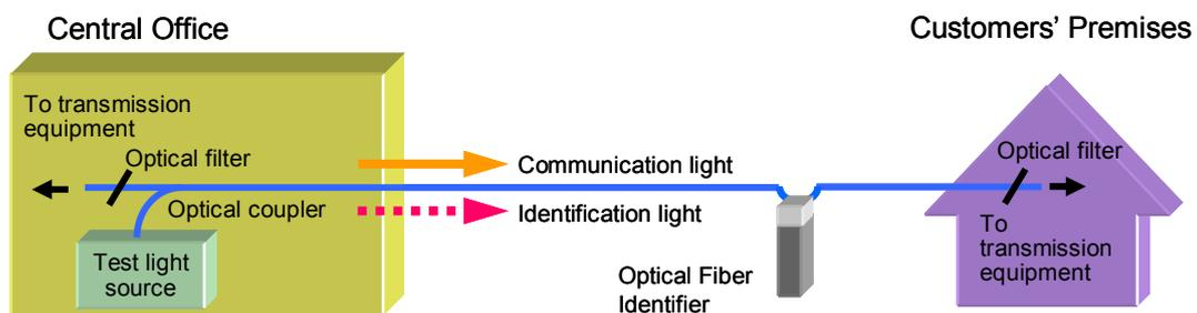
Figure I.1 – Configuration of optical fibre identification
