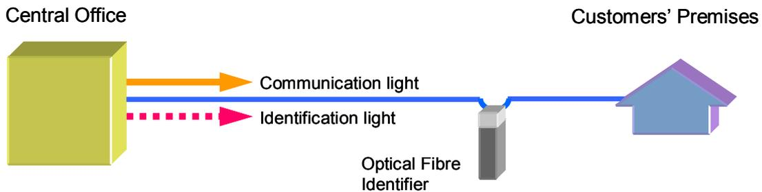
**Figure 1 – Configuration for optical fibre identification**
