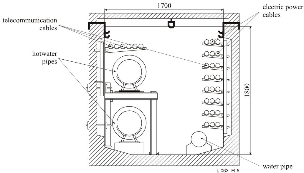
**Figure I.5 – Underground collector**
