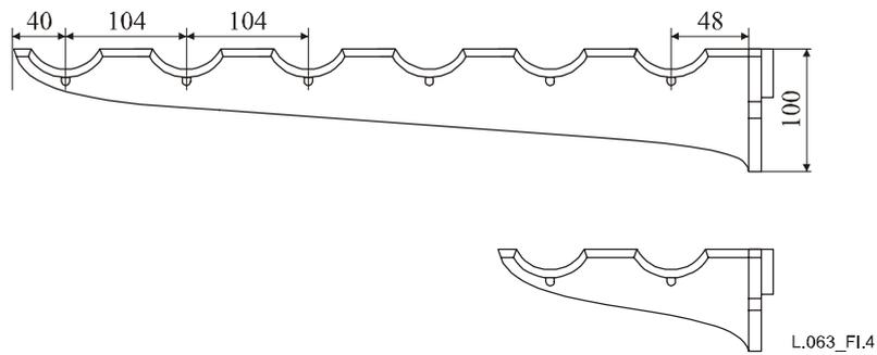
**Figure I.4 – Cable brackets**
