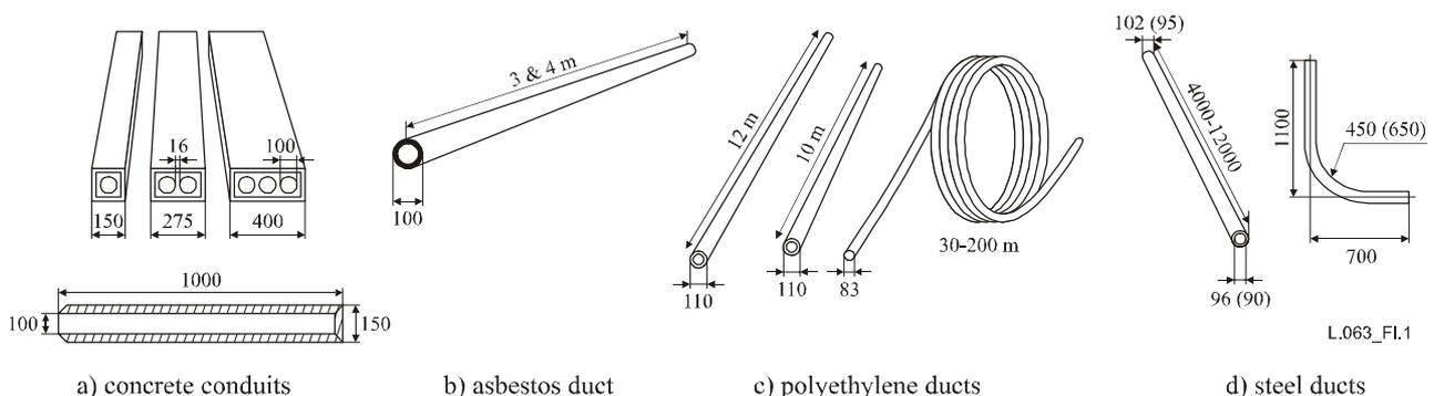
**Figure I.1 – Different types of duct (concrete, asbestos, polyethylene, steel)**
