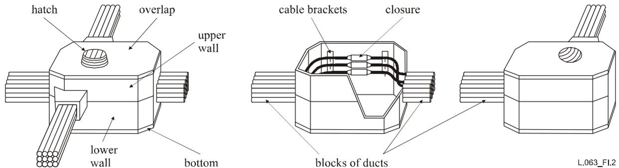
**Figure I.2 – Building blocks of a communication duct**
