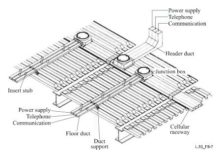
Figure II.7 – Outline of cellular raceway system
