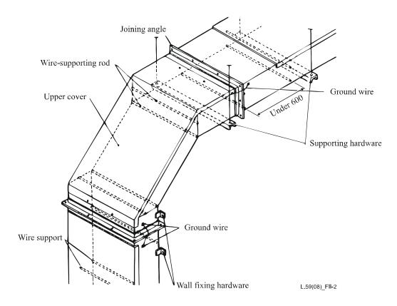
Figure II.2 – Metal duct system
