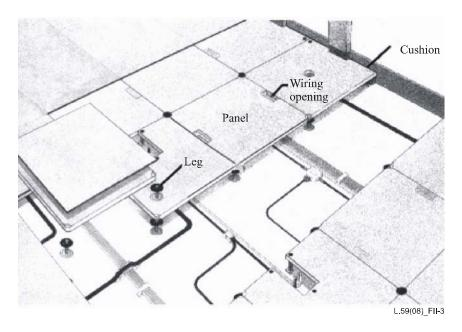
Figure II.3 – Example of simplified access floor system (panel-leg separate type)
