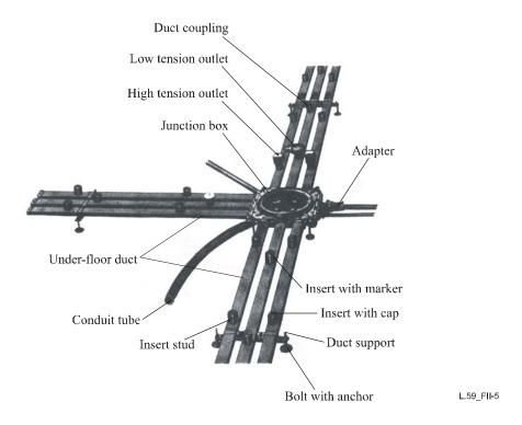
Figure II.5 – Outline of under-floor duct system
