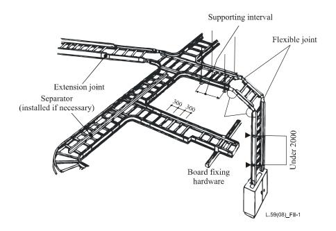
Figure II.1 – Example of ladder cable tray system
