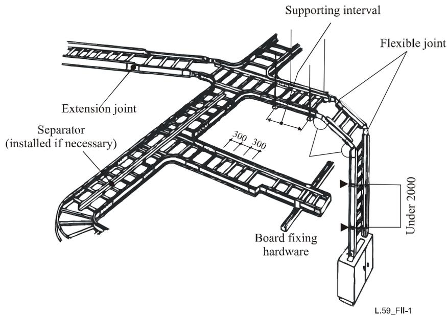
**Figure II.1/L.59 – Example of ladder cable tray system**
