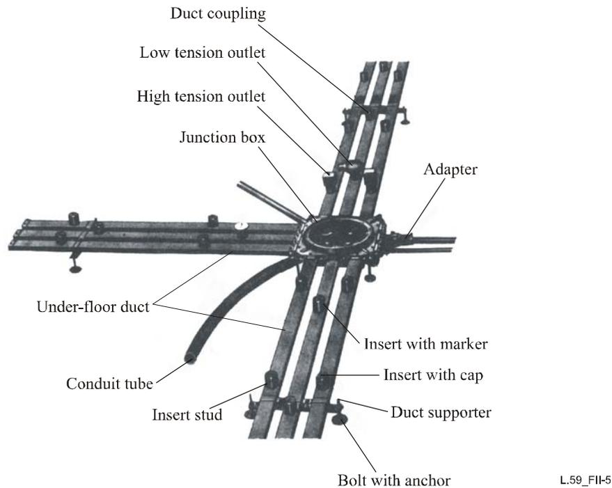
**Figure II.5/L.59 – Outline of under-floor duct system**
