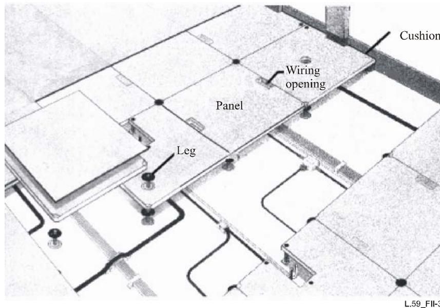
**Figure II.3/L.59 – Example of simplified access floor system (Panel-leg separate type)**
