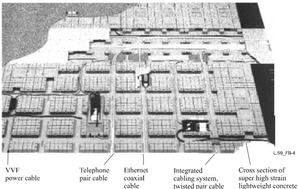
**Figure II.4/L.59 – Example of simplified access floor system (Floor-mounted type)**
