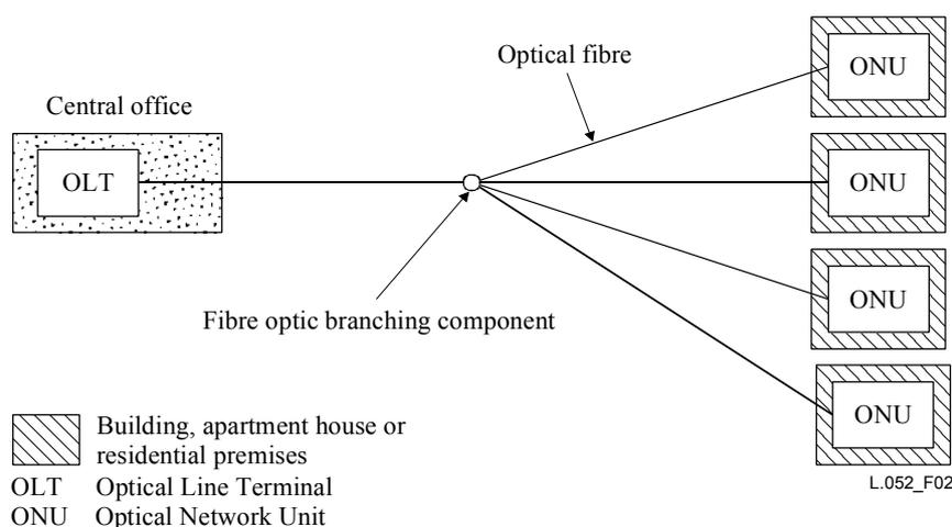
**Figure 2/L.52 – PON configuration using (fibre optic) branching components for an outside plant (with 4 branches)**
