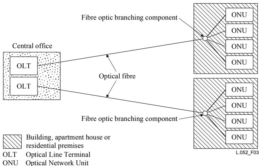
**Figure 3/L.52 – PON configuration using (fibre optic) branching components for a building, apartment house or residential premises (with 4 branches)**
