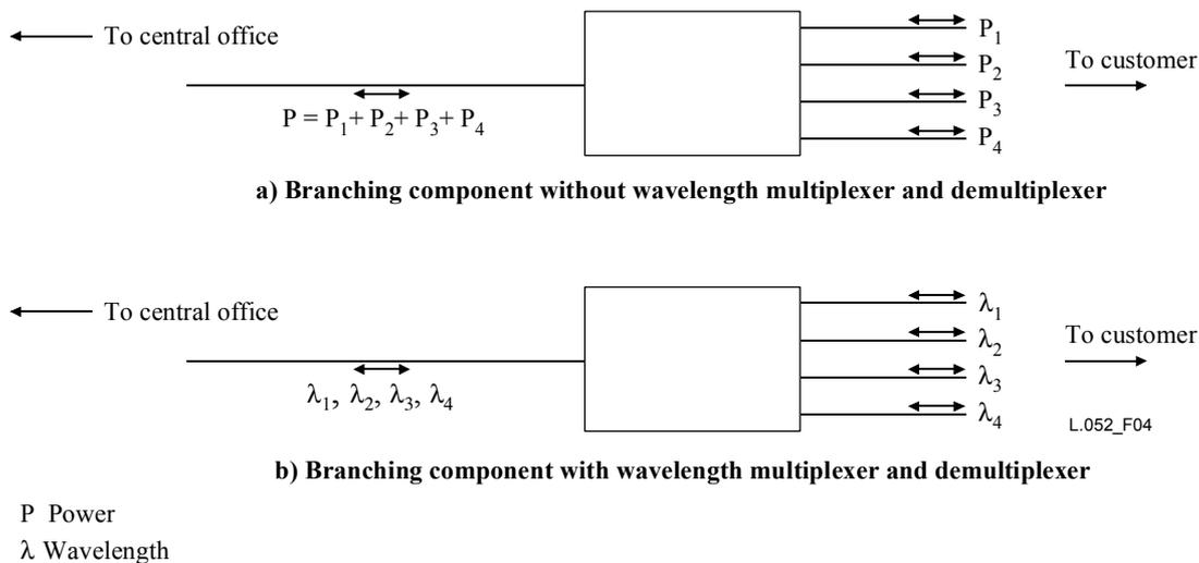
**Figure 4/L.52 – (Fibre optic) branching component**
