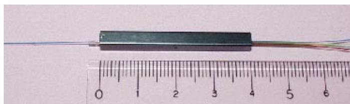
**Figure I.2/L.52 – Photograph of prototype (fibre optic) branching component**
