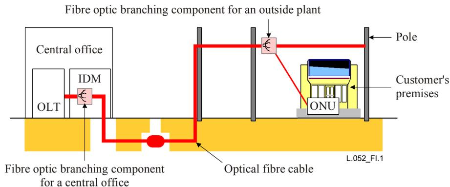
**Figure I.1/L.52 – Configuration of optical fibre network using a (fibre optic) branching component for a central office and an outside plant**
