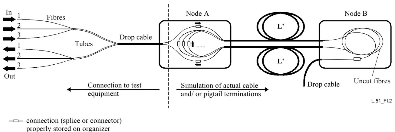
**Figure I.2/L.51 – Storage of uncut single fibre loops**
