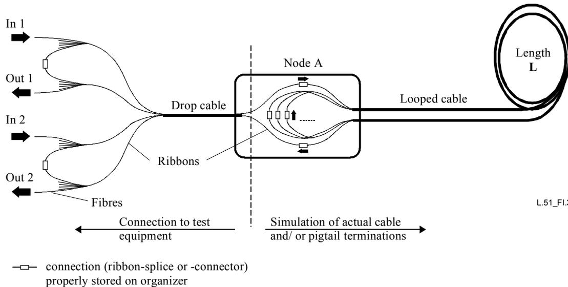
**Figure I.3/L.51 – Storage of ribbon splices or connectors**
