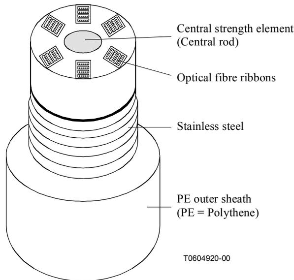
**Figure II.5/L.46 – Configuration of high strength (HS) cable**
