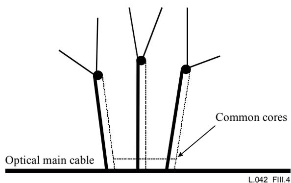
**Figure III.4/L.42 – Link distribution method**
