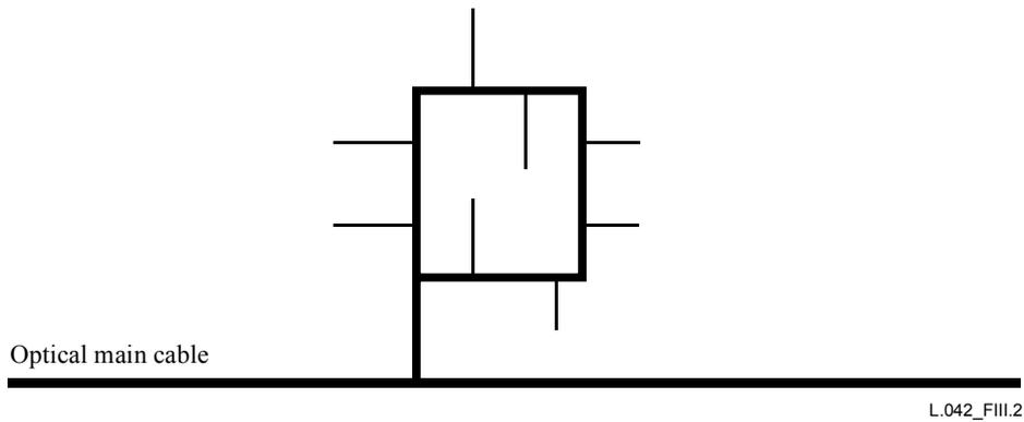
**Figure III.2/L.42 – Loop distribution method**
