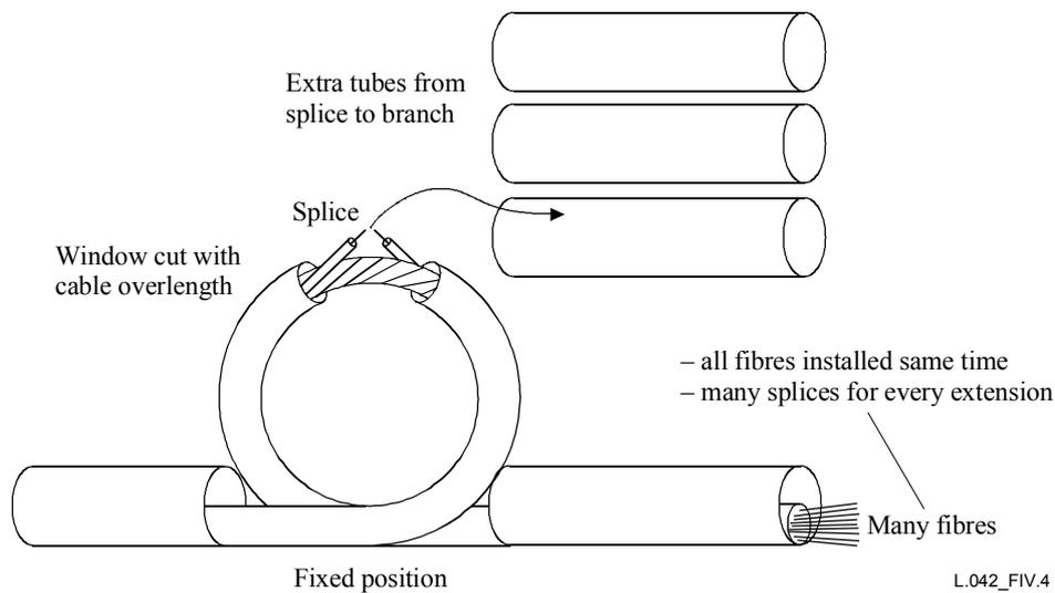
**Figure IV.4/L.42 – A splice-point with cable-overlength when using traditional optical cabling**
