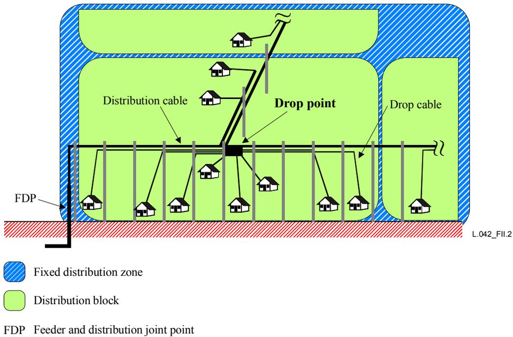
**Figure II.2/L.42 – Distribution block configuration**
