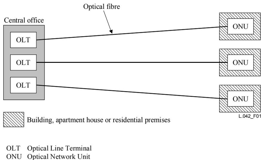
**Figure 1/L.42 – Point-to-point network**
