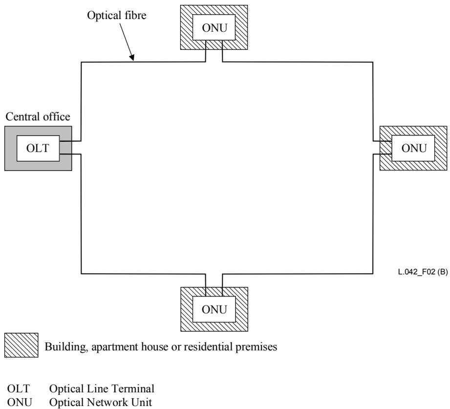
**Figure 2b/L.42 – Ring network (Multiple type)**
