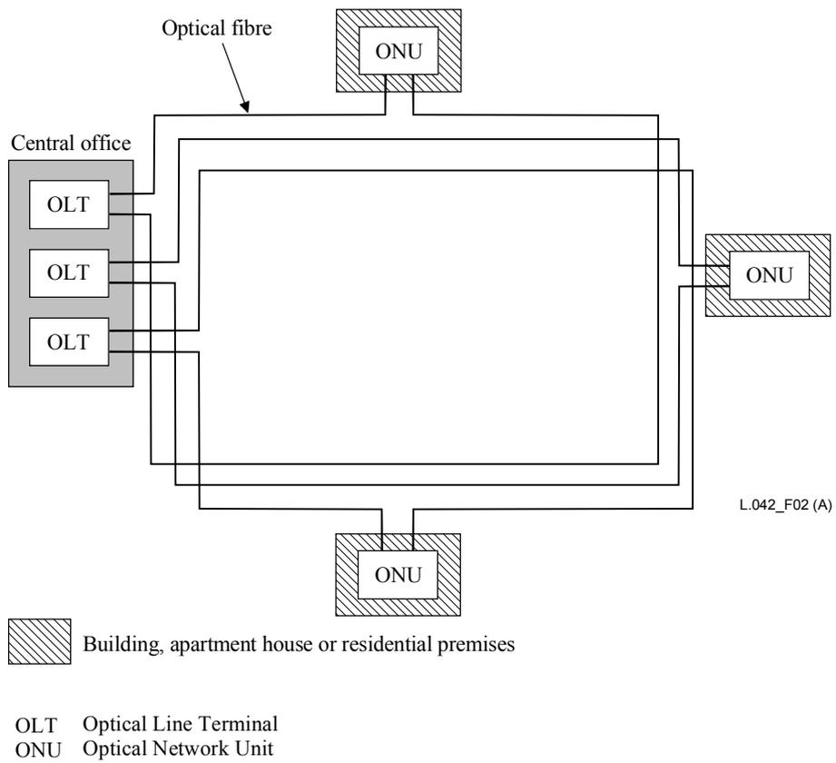
**Figure 2a/L.42 – Ring network (Point-to-point type)**
