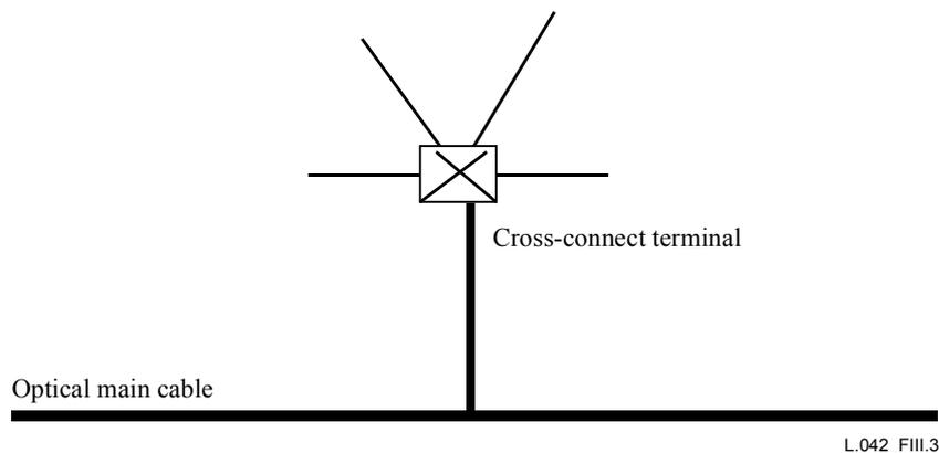
**Figure III.3/L.42 – Cross-connect distribution method**
