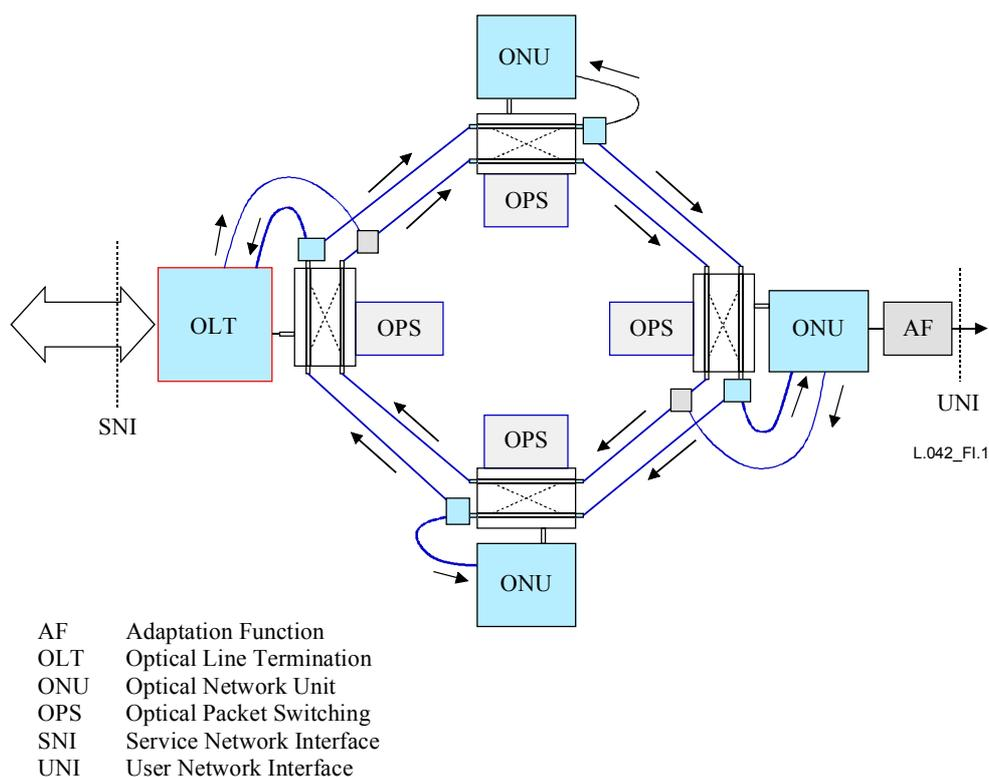
**Figure I.1/L.42 – Ring topology OAN with all-optical add, drop, and route functions**
