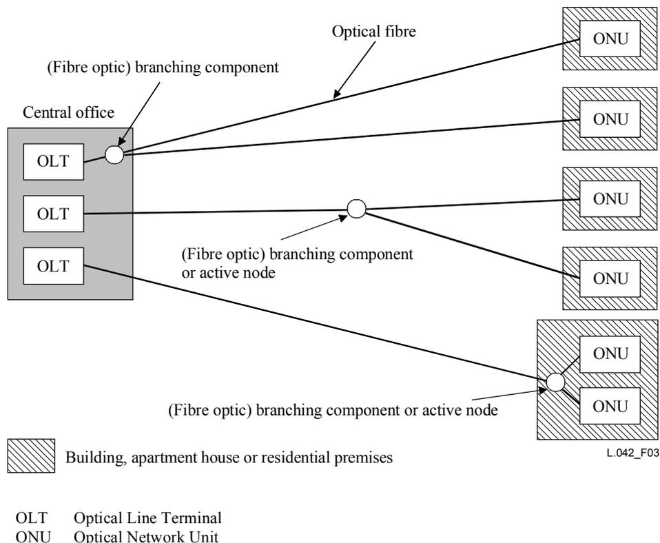
**Figure 3/L.42 – Point-to-multipoint network (in case of 2 branches)**
