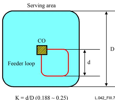
**Figure III.7/L.42 – K, one side length ratio of feeder loop (d) versus the boundary (D) of CO's serving area**
