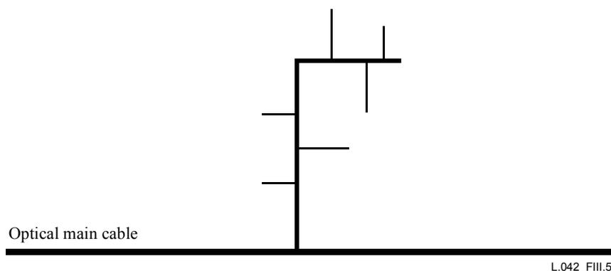
**Figure III.5/L.42 – Non-reduced tree distribution method**
