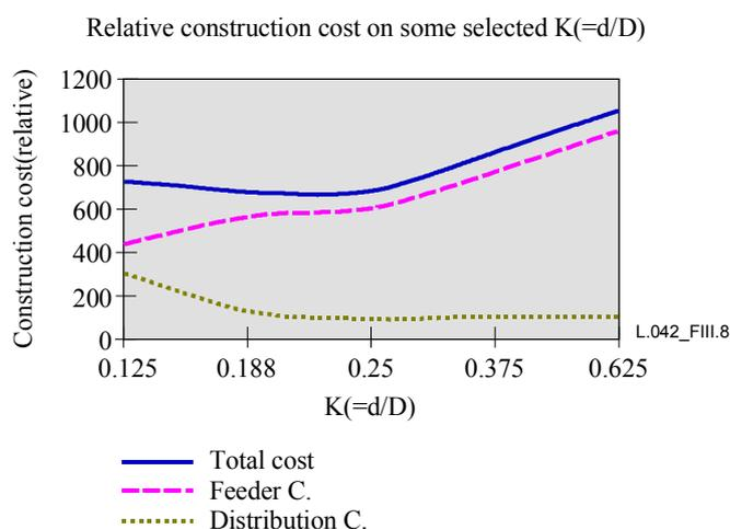
**Figure III.8/L.42 – Relative construction cost on some selected K(=d/D)**
