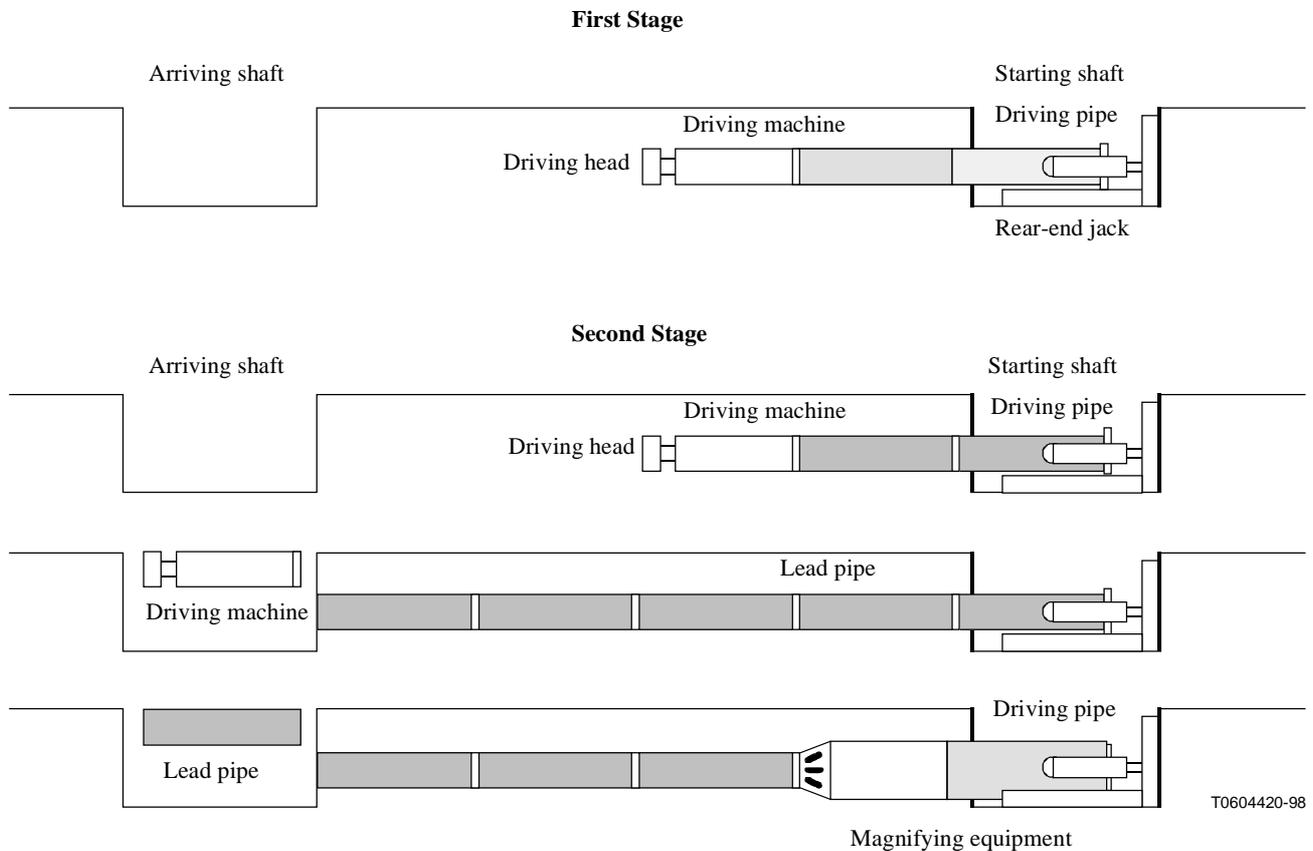
**Figure I.9/L.38 – Difference of first stage and second stage**
