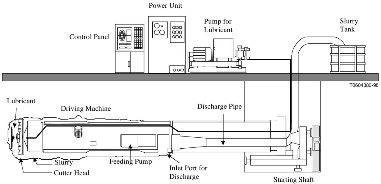
**Figure I.6/L.38 – Example of slurry pressure balanced method**
