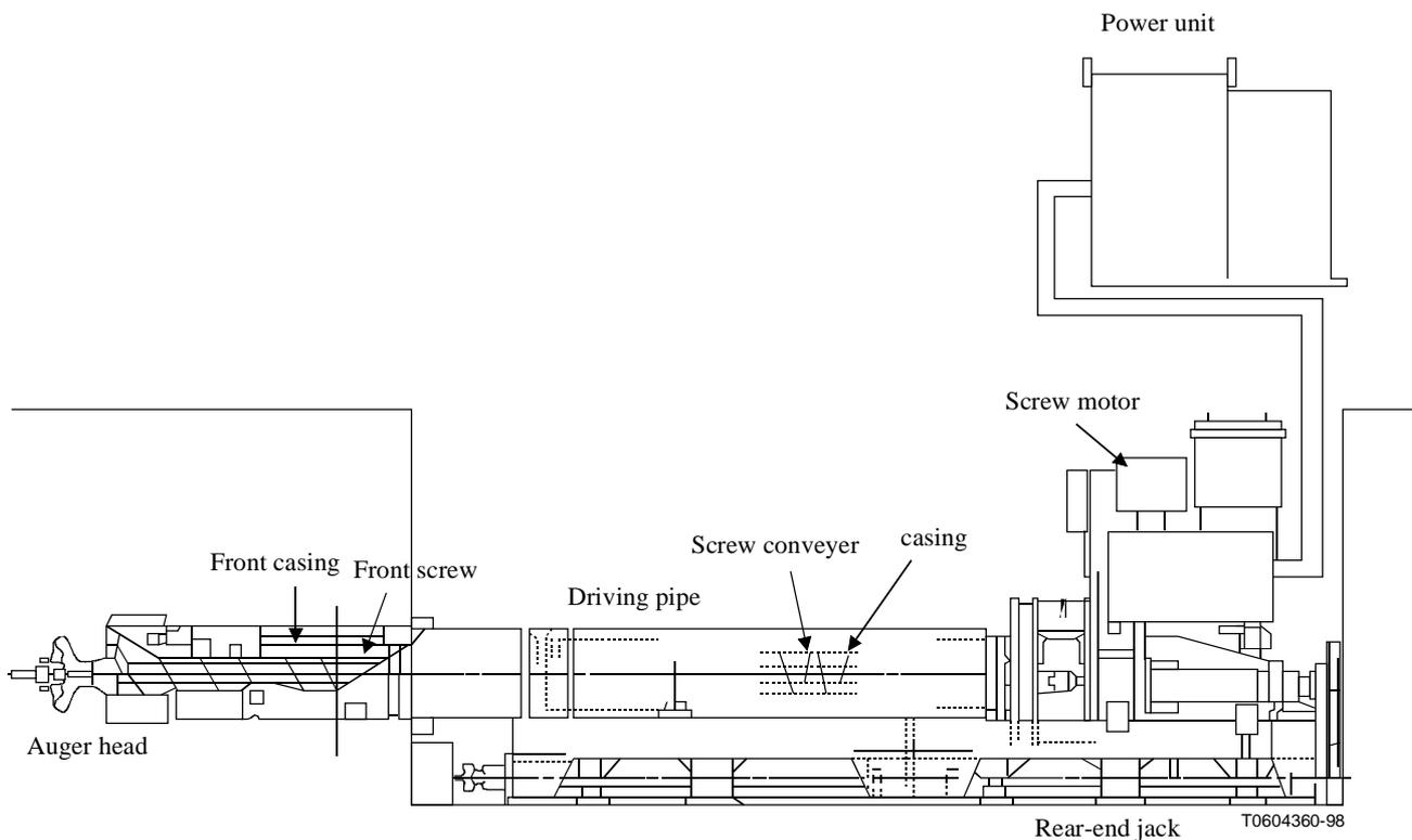
**Figure I.4/L.38 – Example of auger excavation method**
