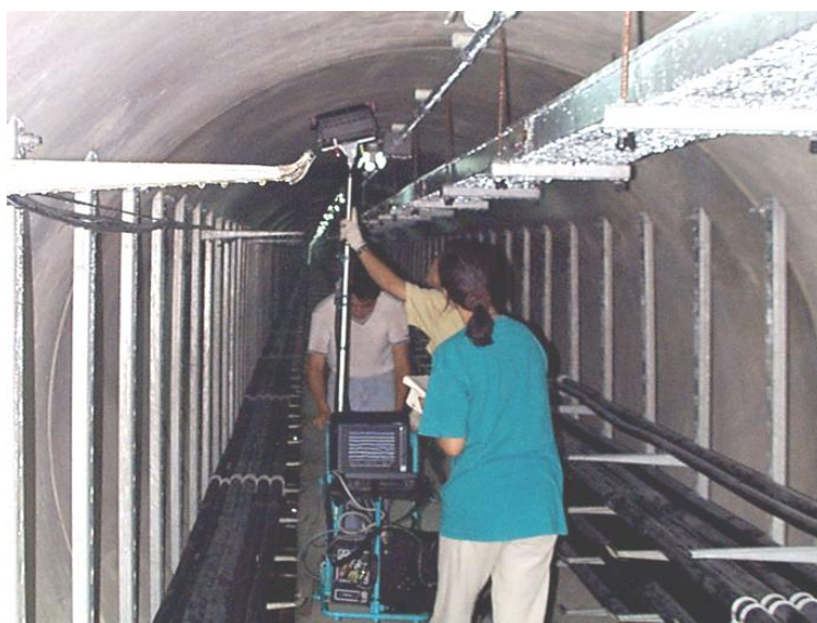
Figure I.4 – Tunnel lining inspection using GPR
