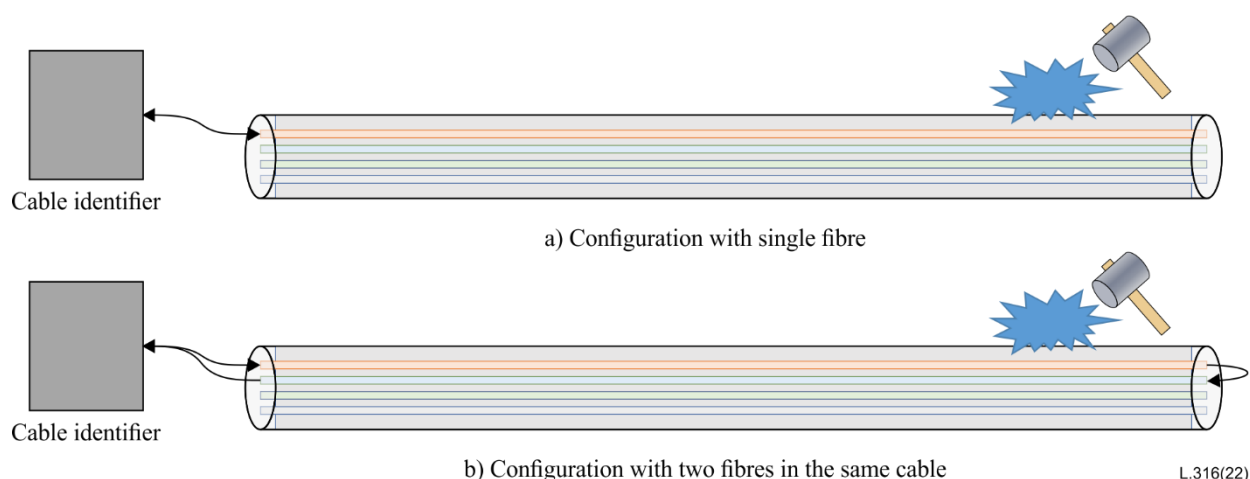
Figure 2 – Interferometry-based cable identification
