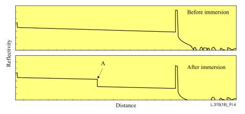
Figure I.4 – OTDR trace before and after water penetration
