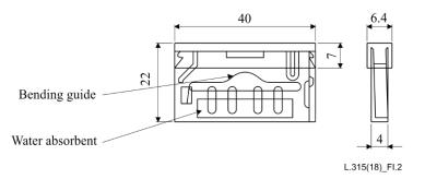
Figure I.2 – Structure of the water submersion-detecting sensor
