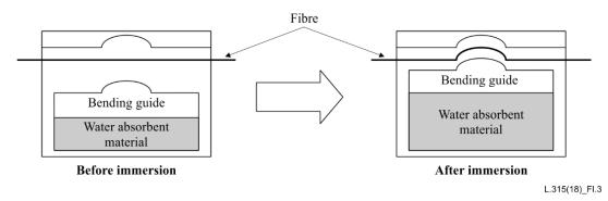
Figure I.3 – Fibre bending after water absorption
