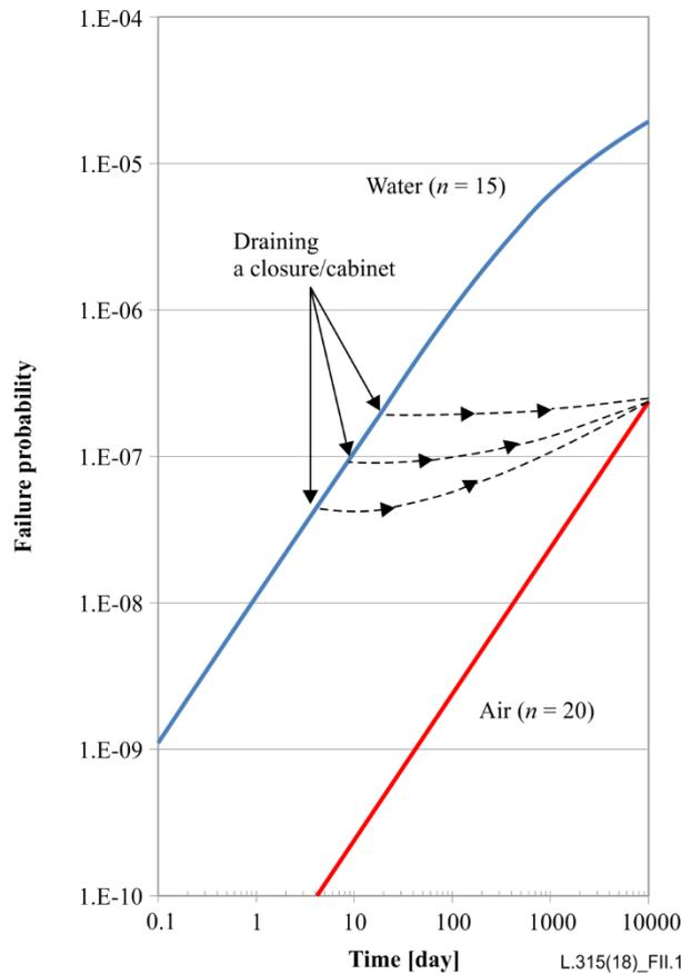
**Figure II.1 – Failure probabilities of a 3-meter optical fibre loosely stored with a 20-mm bending radius**
