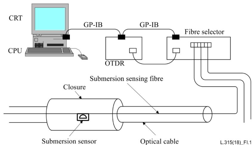
Figure I.1 – Fibre optic water submersion-detecting sensor
