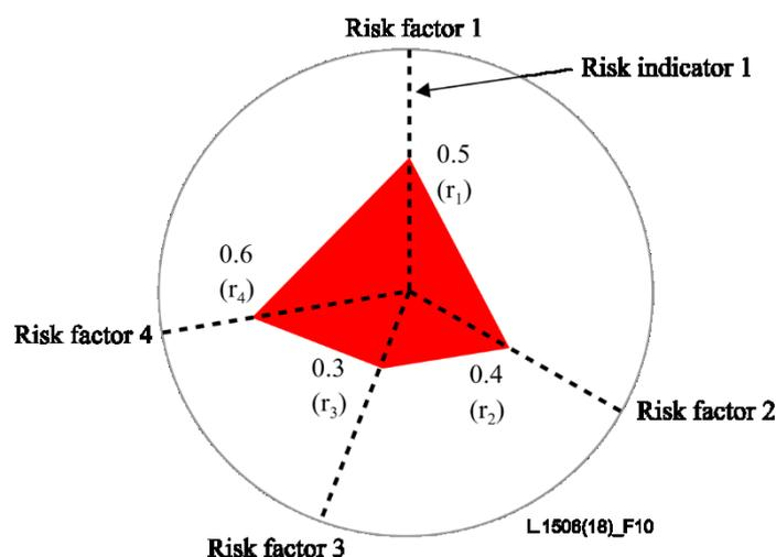
**Figure 10 – Example of a weighted spider web chart for a weighted surface measure overall performance calculation**
