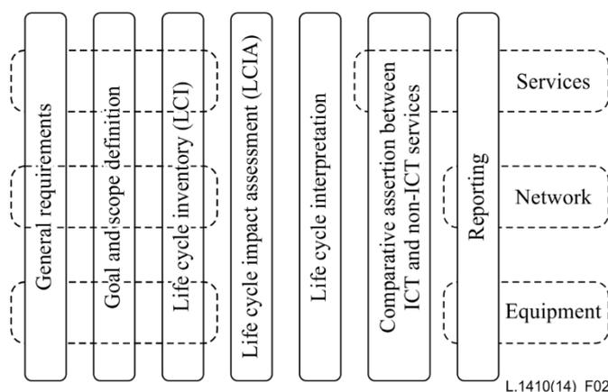
**Figure 2 – Structure of LCA methodology specification for ICT goods, networks and services**
