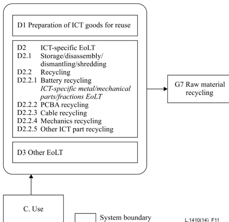
**Figure 11 – The system boundary of goods EoLT in LCA of ICT goods**
