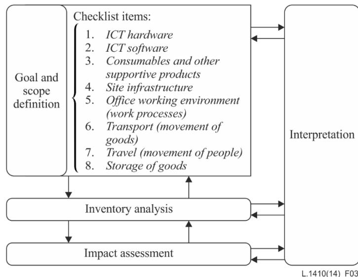
**Figure 3 – Framework of Part I of this Recommendation**
