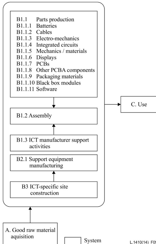
**Figure 9 – The system boundary of Production in LCA of ICT goods**
