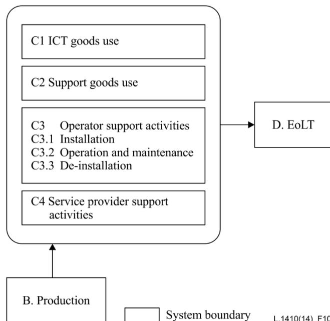
**Figure 10 – The system boundary of use in LCA of ICT goods**
