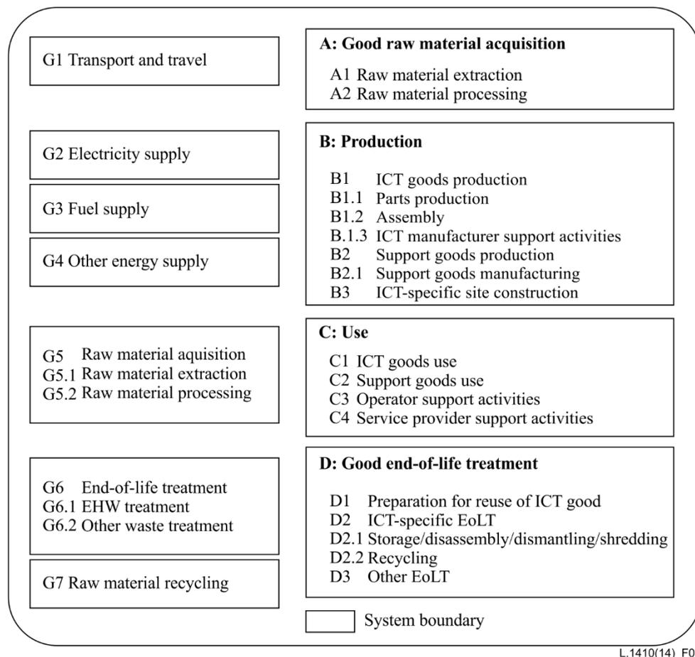
**Figure 7 – The system boundary of the product system for LCAs of ICT goods, networks or services**
