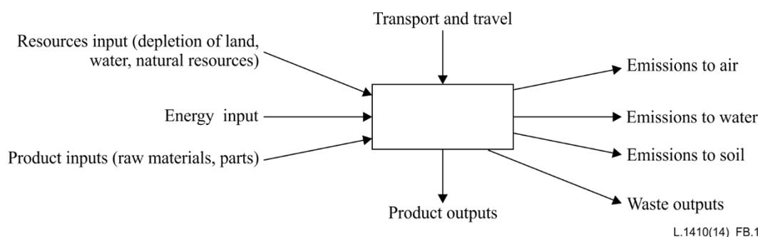
**Figure B.1 – The generic unit process model**
