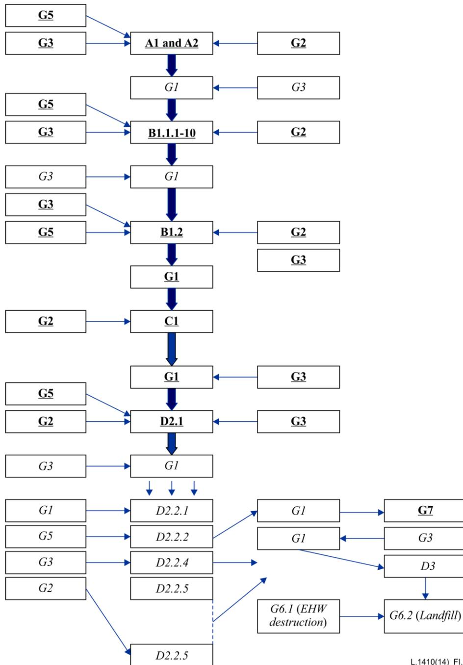
**Figure I.2 – The system boundary of the product system for LCA of the mobile phone showing connections with generic processes**
