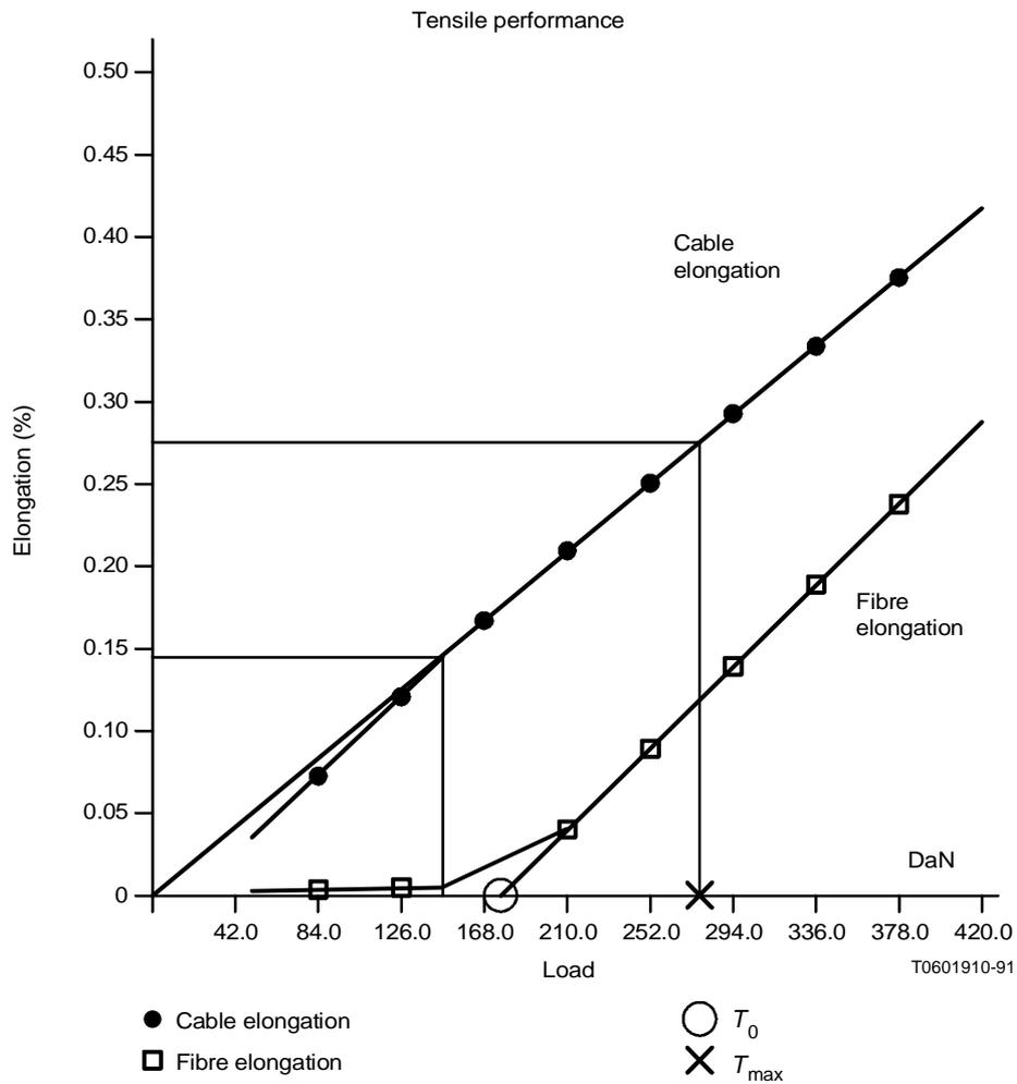
Note –  $T_0$  corresponds to the load at which the fibre becomes under strain.
