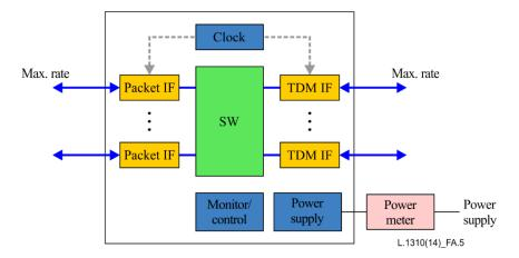
Figure A.5 – Example of maximum component configuration for measuring P<sub>max</sub>
