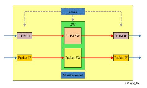
Figure A.1 – Converged packet optical equipment I configuration (Model I)
