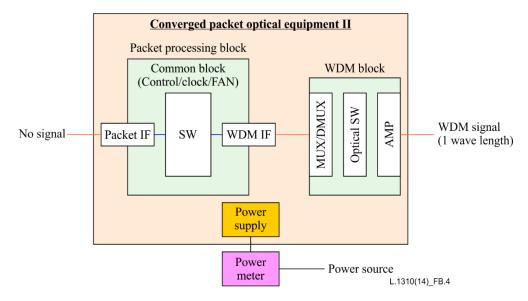
Figure B.4 – Example of minimum component and path configuration for measuring Pidle
