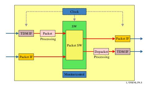
Figure A.3 – Converged packet optical equipment I configuration (Model III)
