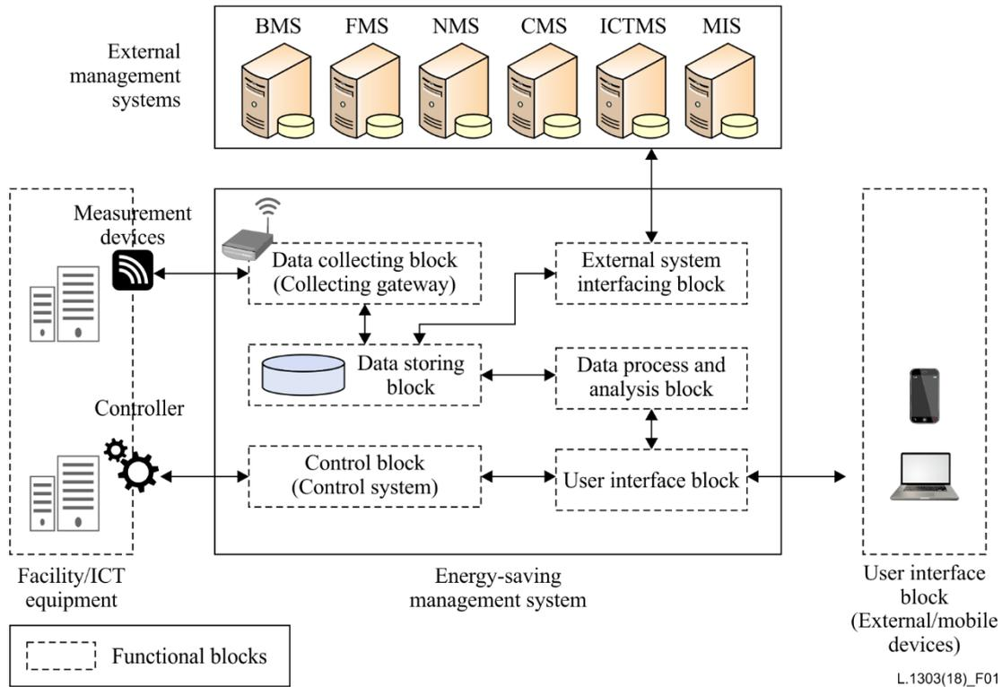
**Figure 1 – Functional block diagram of the ESMS**
