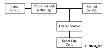
Figure II.1 – Schematic of supercapacitor unit for fibre to the x application
