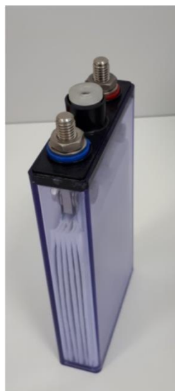
Internal structure of Nickel-Zinc battery (similar to other Nickel-Based battery)
