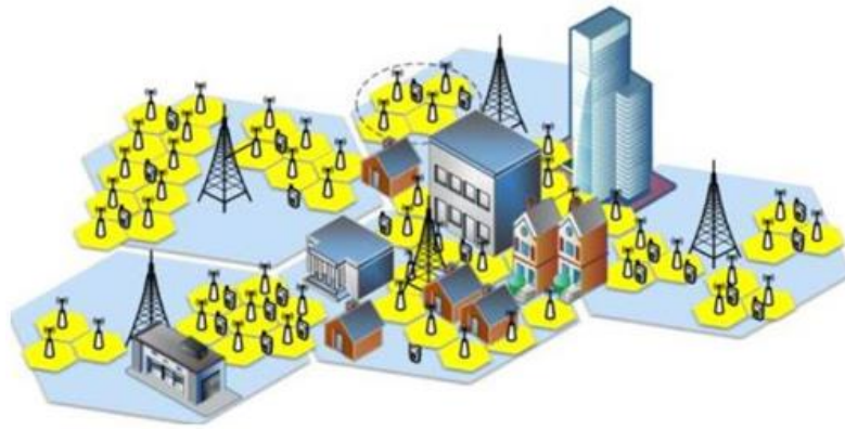
Figure 2 (a) – Deployment mode of the 5G base station
