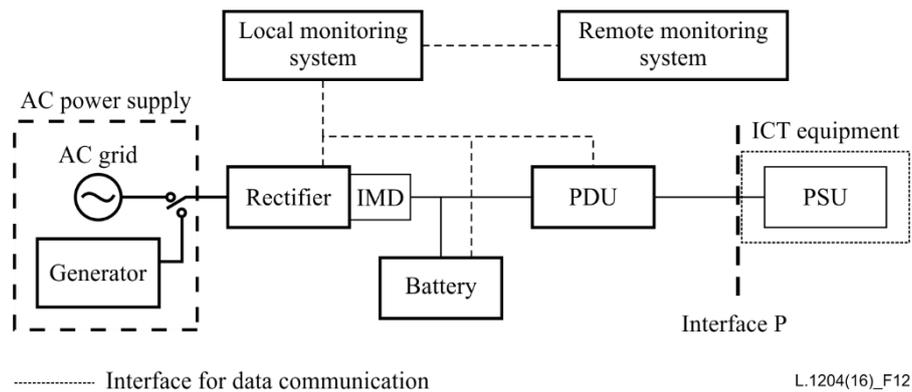
**Figure 12 – Monitoring entities in a typical power feeding system of up to 400 VDC**
