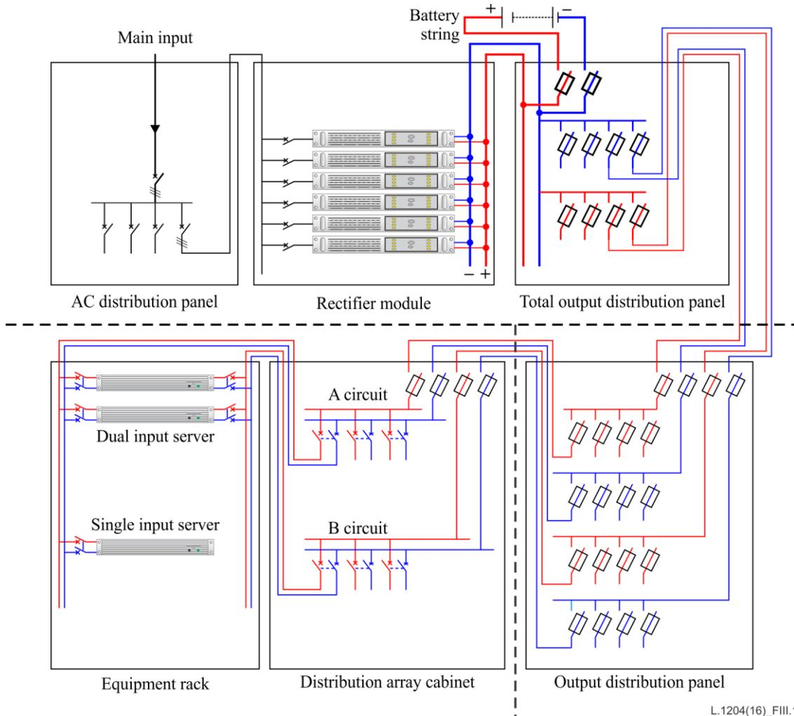
**Figure III.1 – Three-level distribution structure**
