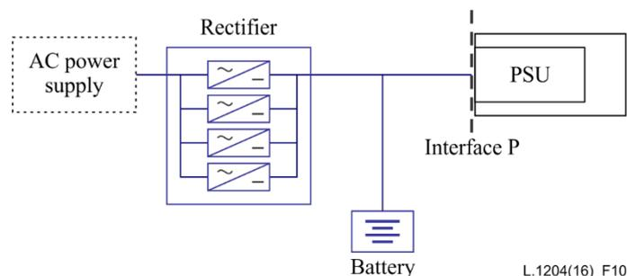
**Figure 10 – Basic configuration of rectifier**
