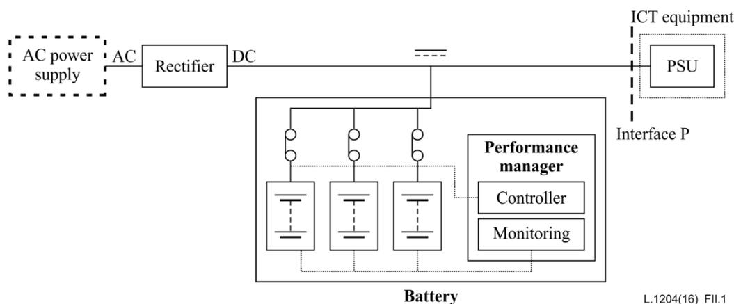
Figure II.1 – Battery configuration with performance manager
