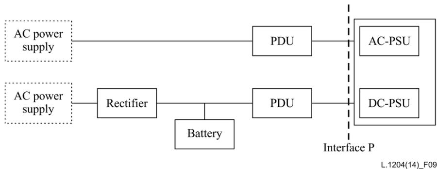
**Figure 9 – AC and DC power feeding system configuration from two independent grids for dual-PSU ICT equipment**
