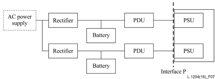
**Figure 7 – System configuration with redundant rectifiers and DC distributions for the redundant input of ICT equipment**
