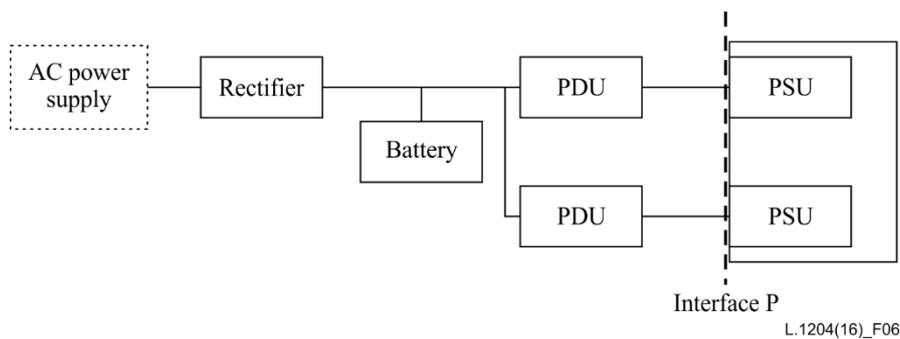
**Figure 6 – System configuration with redundant PDUs for the redundant input of ICT equipment**
