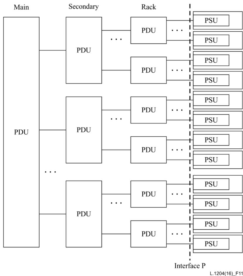
**Figure 11 – Example configuration of multi-level PDU**
