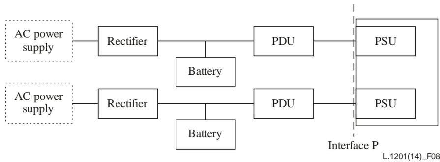
**Figure 8 – System configuration with end-to-end redundancies of power feeding systems for the redundant inputs of ICT equipment**
