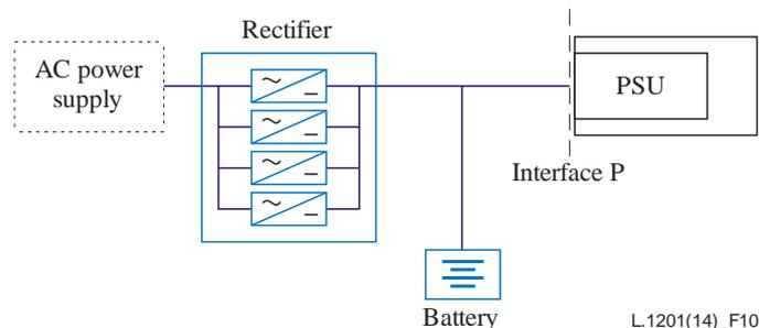
**Figure 10 – Basic configuration of rectifier**
