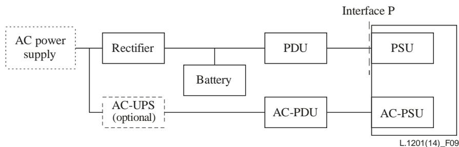
**Figure 9 – AC and 'up to 400 VDC' power feeding system configuration for redundant inputs of ICT equipment**
