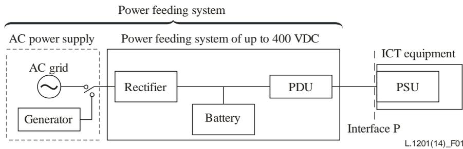
**Figure 1 – Typical power feeding system configuration integrating a power feeding system of up to 400 VDC**
