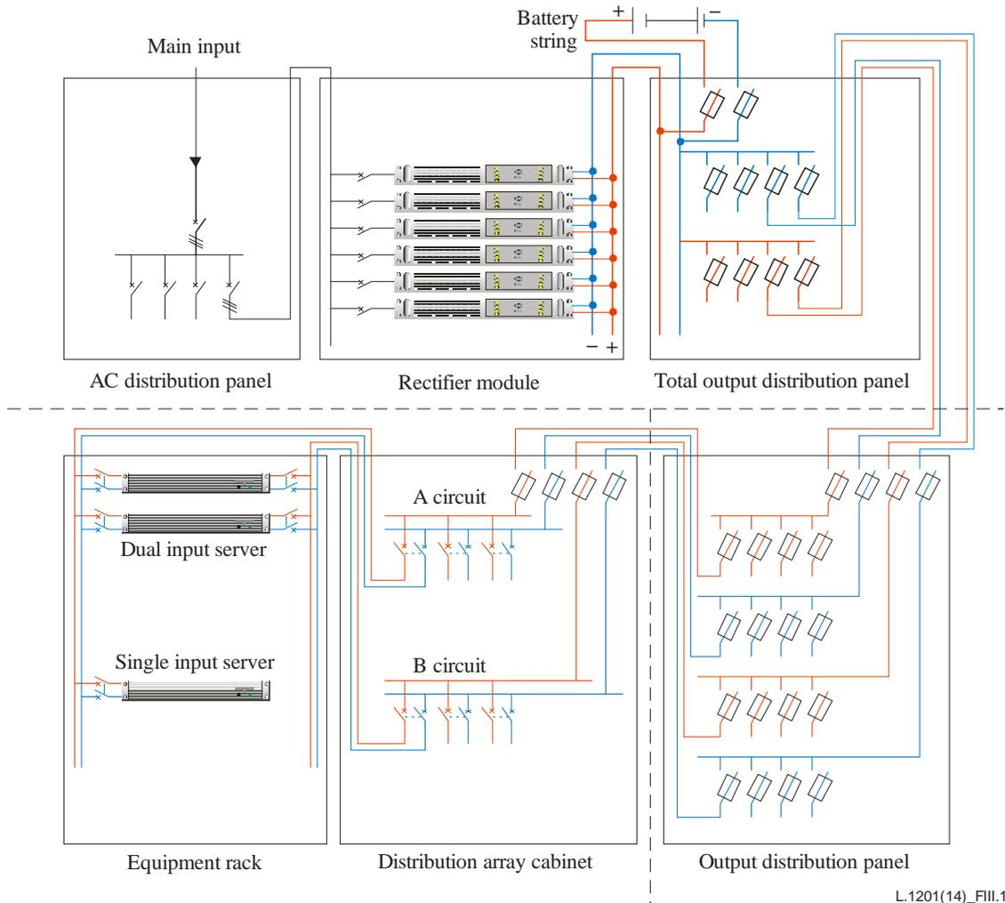
**Figure III.1 – Three-level distribution structure**
