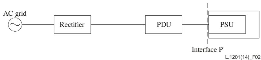
**Figure 2 – Simplest system configuration of up to 400 VDC power feeding**
