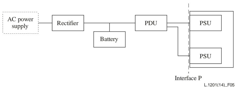
**Figure 5 – System configuration with the redundant input of ICT equipment**
