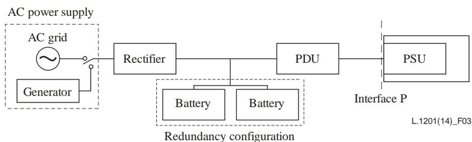
**Figure 3 – Power feeding system of up to 400 VDC with backup solution**
