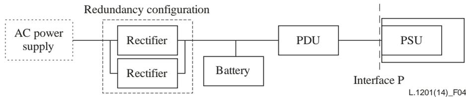
**Figure 4 – Example of a system configuration with redundant rectifiers**
