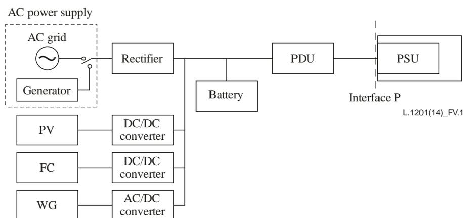
Figure V.1 – Direct connection in DC of PV, FC or WG generators to a DC power feeding
