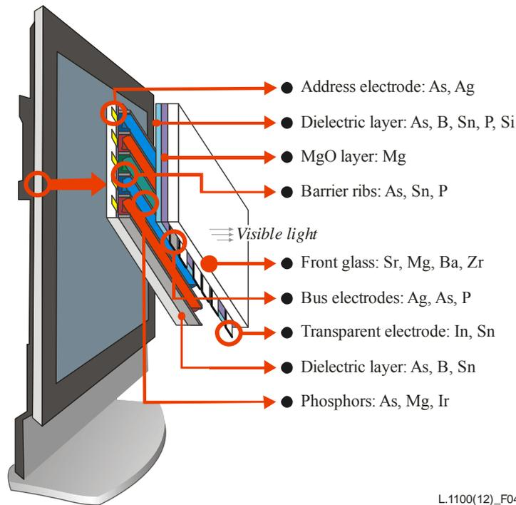
**Figure 4 – Rare metals contained in an LCD**
