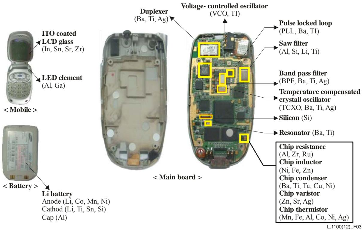
**Figure 3 – Rare metals contained in a mobile phone**
