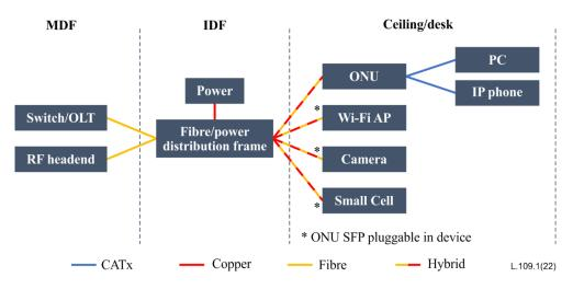
Figure 6-1 – Power and data delivery networking based on OEHC
