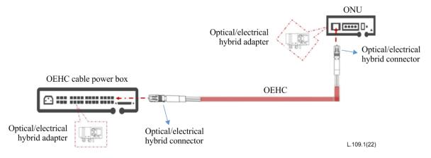
Figure I.3 – Power supply networking for the hybrid cable ONU
