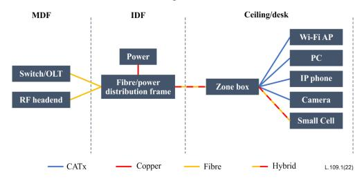
Figure 6-2 – OEHC application on the fibre and power to the zone and the small cell scenario
