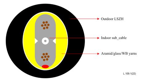
Figure I.2 – Indoor/outdoor optical/electrical hybrid cable
