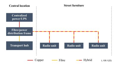
Figure 6-3 – Centralised fibre connectivity and power delivery network based on multi fibre OEHC
