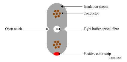
Figure I.1 – Indoor optical/electrical hybrid cable
