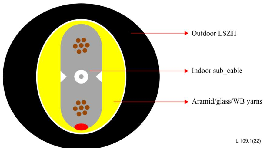
Figure I.2 – Indoor/outdoor optical/electrical hybrid cable
