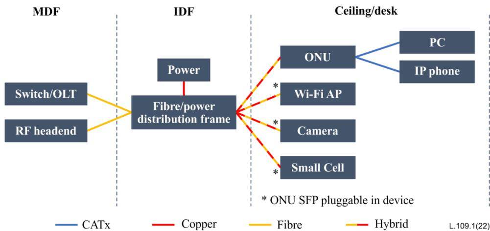
**Figure 6-1 – Power and data delivery networking based on OEHC**
