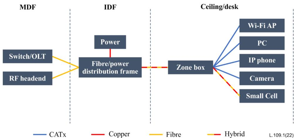
**Figure 6-2 – OEHC application on the fibre and power to the zone and the small cell scenario**
