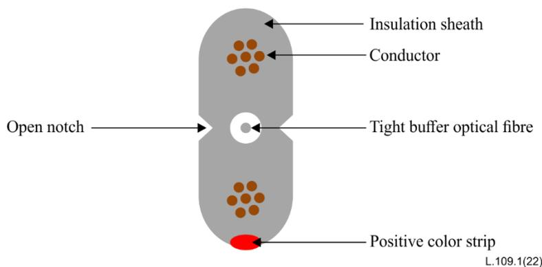
Figure I.1 – Indoor optical/electrical hybrid cable
