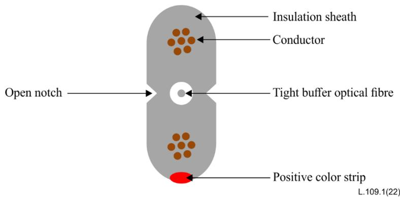
Figure I.1 – Indoor optical/electrical hybrid cable
