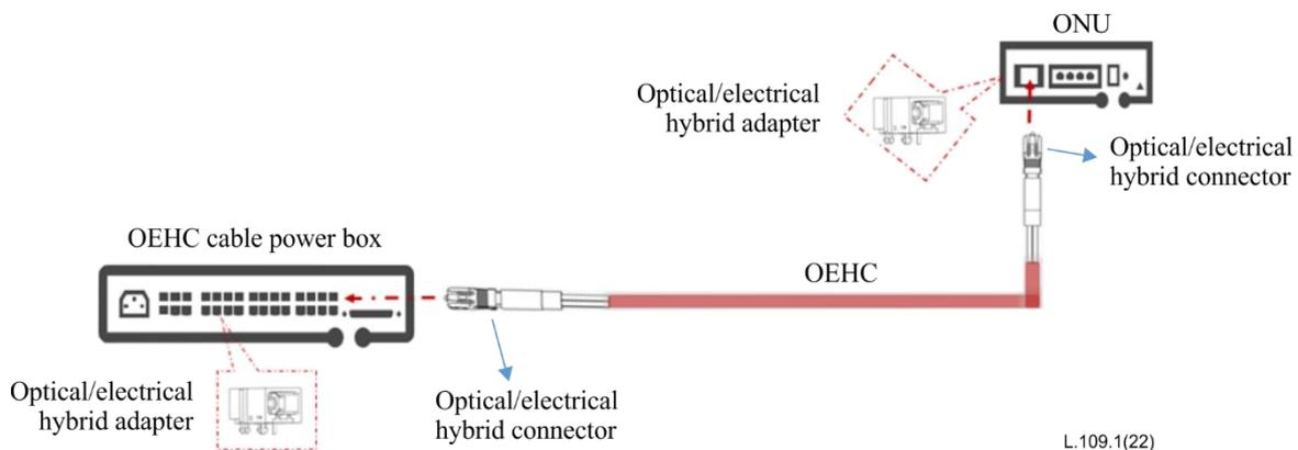
**Figure I.3 – Power supply networking for the hybrid cable ONU**
