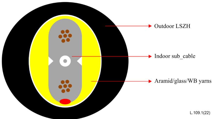
Figure I.2 – Indoor/outdoor optical/electrical hybrid cable
