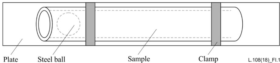
**Figure I.1 – Test set-up for microduct inner clearance verification**
