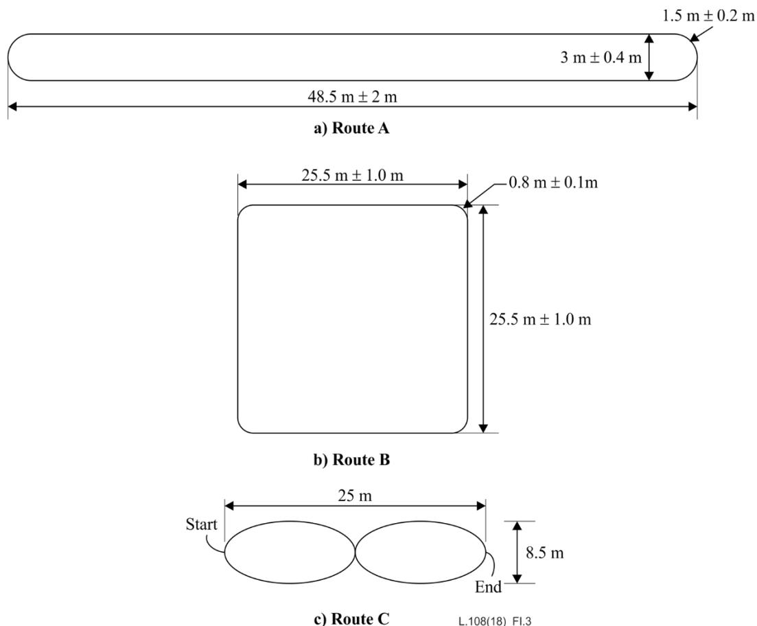
**Figure I.3 – Test set-up for blowing performance in the field (simulated)**
