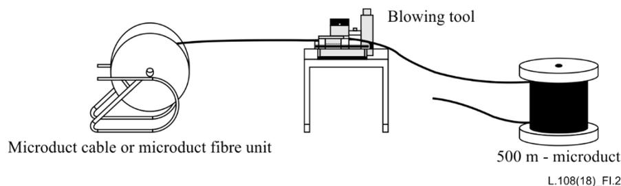
**Figure I.2 – Test set-up for blowing performance on drum**
