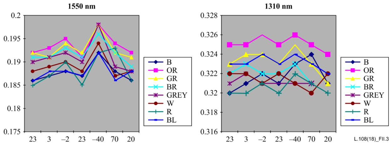
**Figure II.3 – Largest attenuation values in each loose tube at different temperature points**
