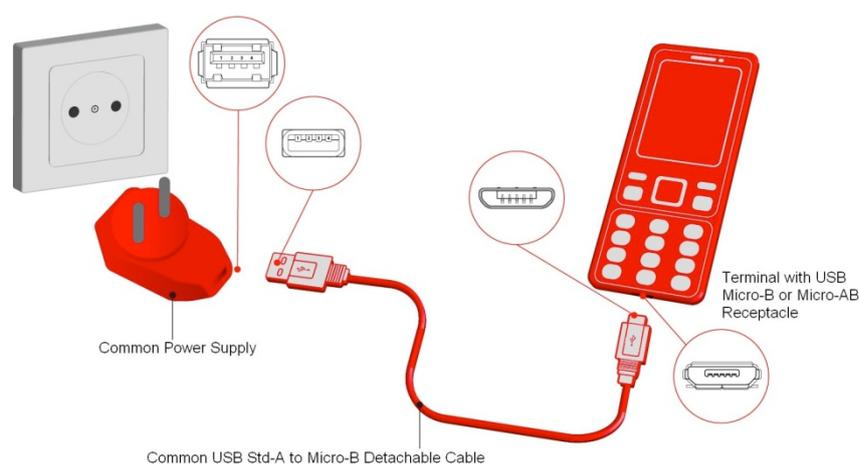
**Figure II.1 – Common charging and local data connectivity**
