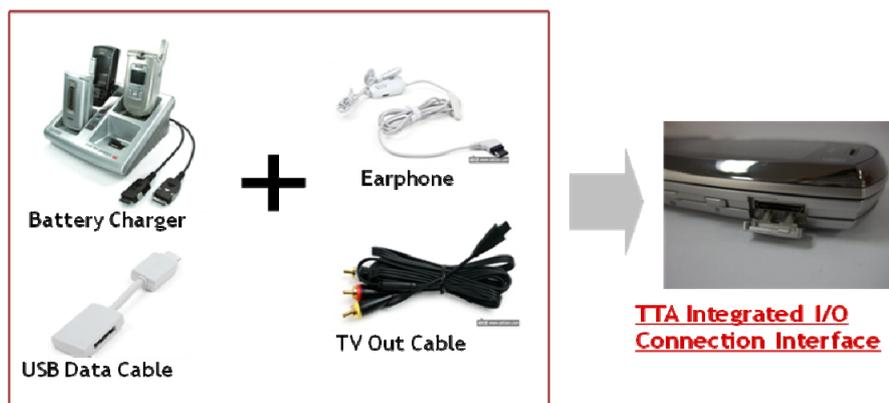
**Figure IV.2 – Integrated I/O connection interface**
