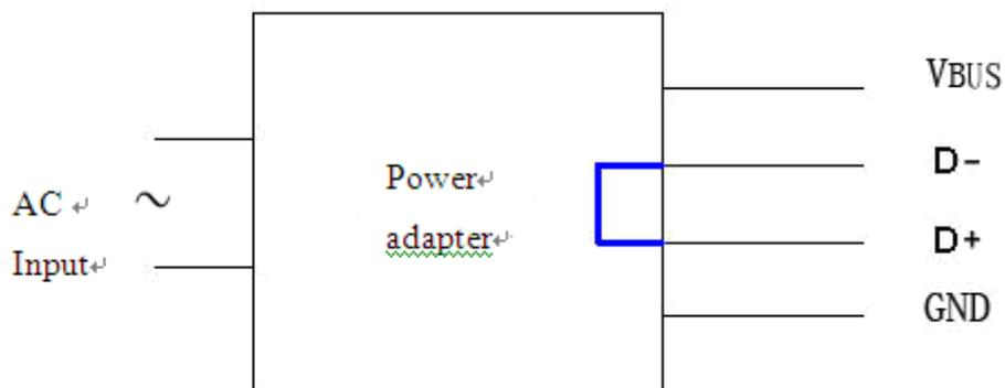
**Figure III.2 – The D+ and D– signal line in the power adapter**
