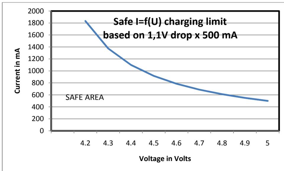
**Figure V.1 – Power adapter safe output characteristic for compatibility with existing phones rechargeable by standard USB plug (5 V × 500 mA)**
