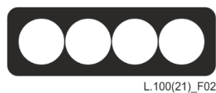
Figure 2 – Cross-section of a typical encapsulated ribbon
