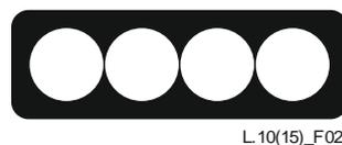
**Figure 2 – Cross-section of a typical encapsulated ribbon**
