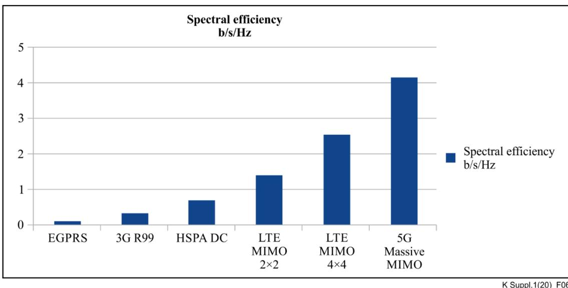
**Figure 6 – Comparison of the mobile systems efficiency**
