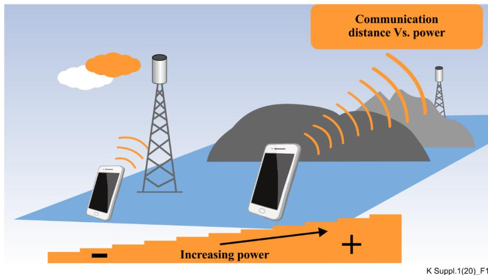
**Figure 13 – Distance from base station and increasing phone power (the + indicates higher power from a mobile phone is required)**
