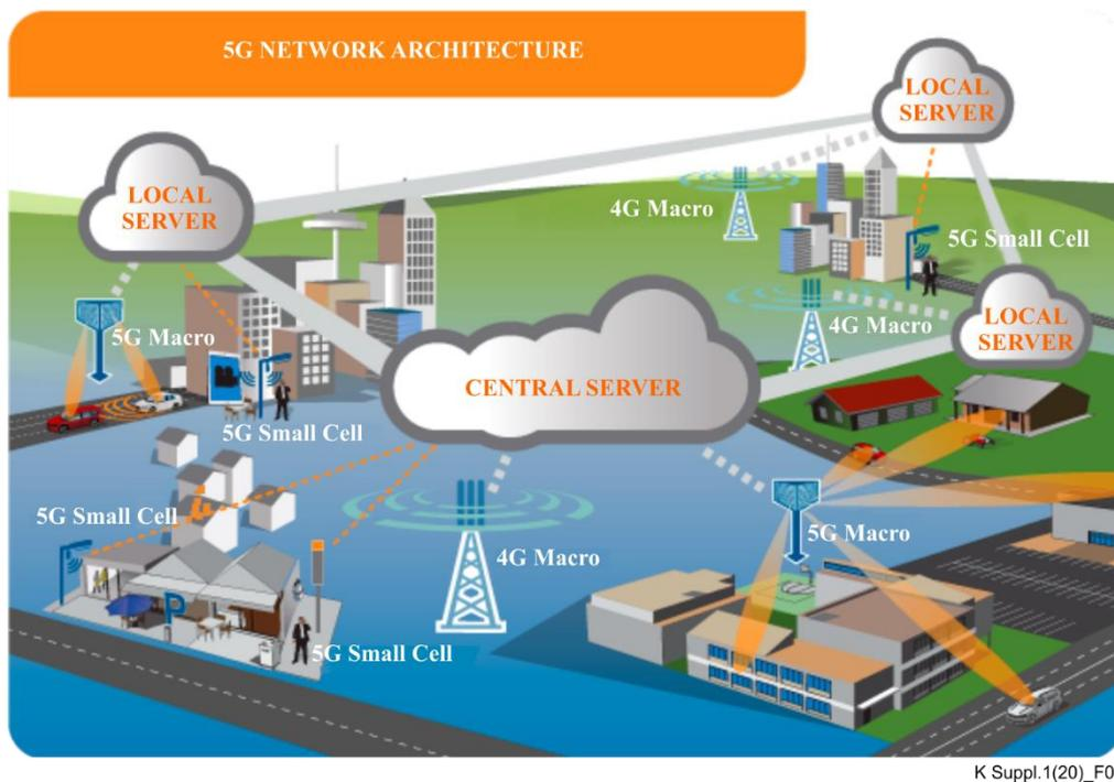
**Figure 9 – 5G network architecture illustrating 5G and 4G working together, with central and local servers providing faster content to users and low latency applications**
