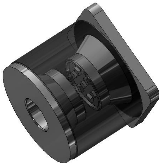
Figure 1 – "See-through" view of a surface mount two-electrode GDT
