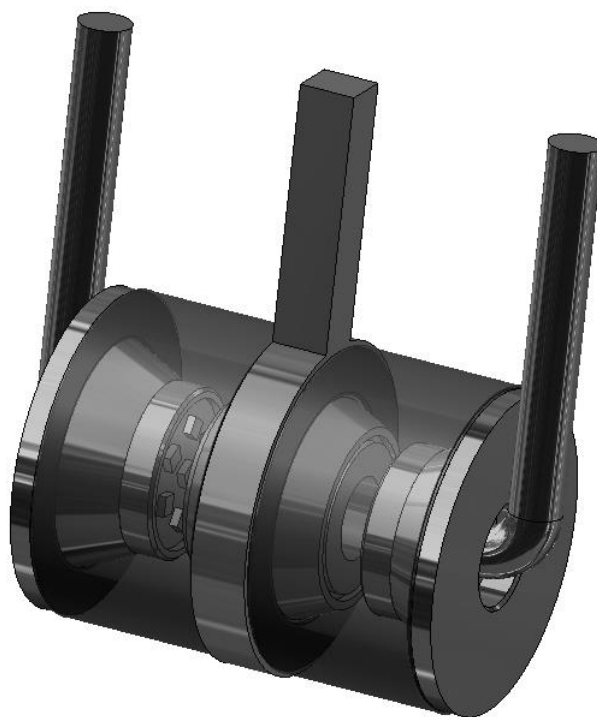
Figure 3 – "See-through" view of a leaded three-electrode GDT
