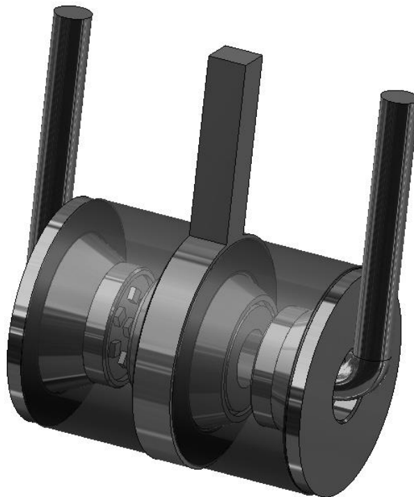
Figure 3 – "See-through" view of a leaded three-electrode GDT
