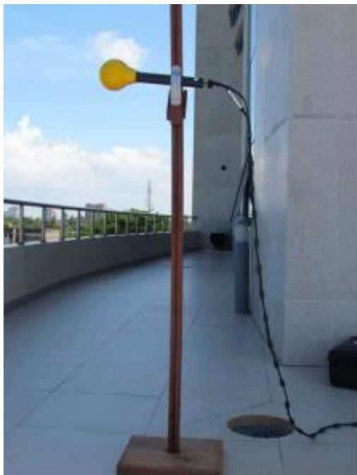
Figure II.9 – Narda probe fixed on a wooden stand
