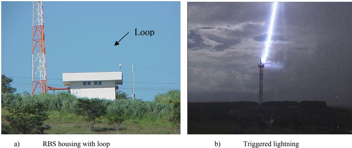
**Figure I.7/K.67 – Test set-up for induced current into a closed loop**
