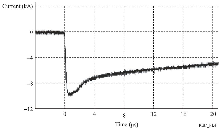
**Figure I.4/K.67 – Triggered lightning current**
