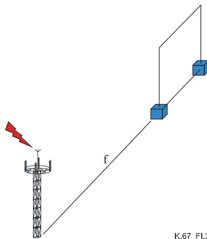
Figure I.3/K.67 – Test set-up for induced voltage into an open loop
