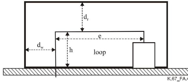
**Figure A.4/K.67 – Lightning strokes to the structure: Grid-like spatial shield LPS**
