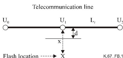
**Figure B.1/K.67 – Reference configuration for surge evaluation induced by lightning near the line**
