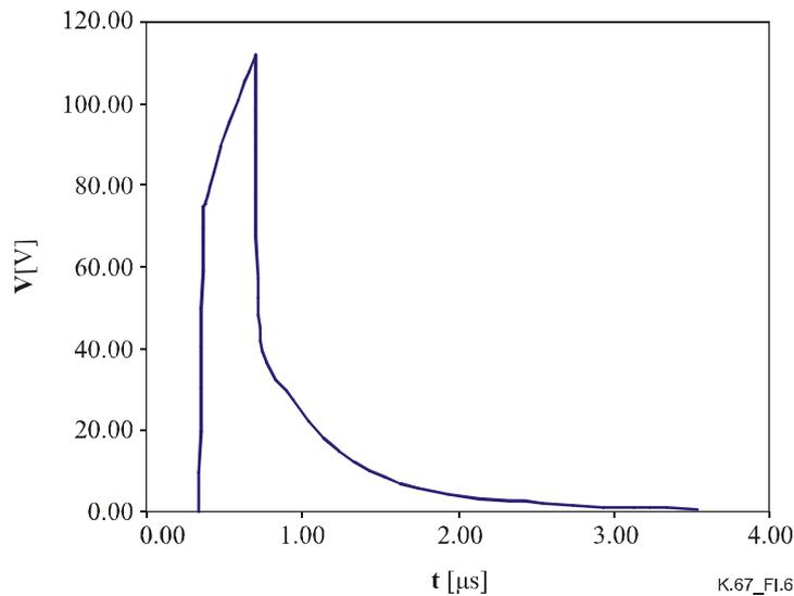
**Figure I.6/K.67 – Voltage wave calculated with from Rusck's model**
