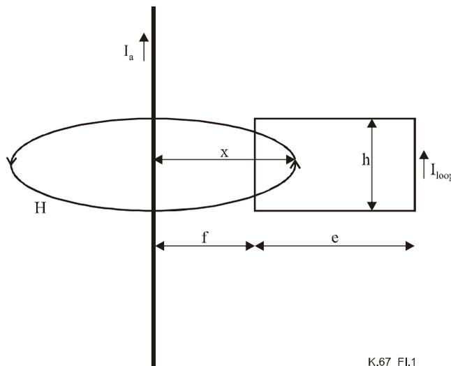
**Figure I.1/K.67 – Induction into a loop**
