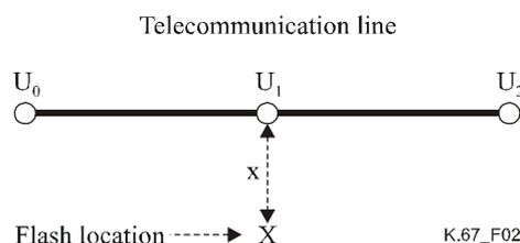
**Figure 2/K.67 – Reference configuration for surge evaluation induced by a lightning near the line (worst case)**
