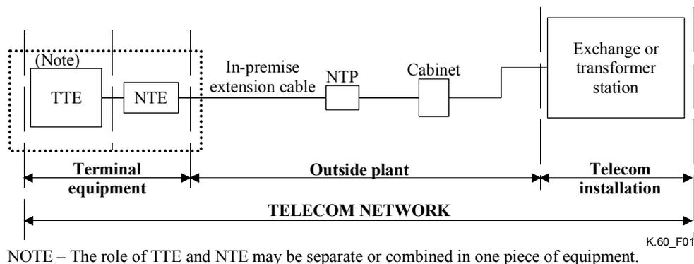
**Figure 1/K.60 – Diagram showing alignment of definitions to a typical telecommunication access network**
