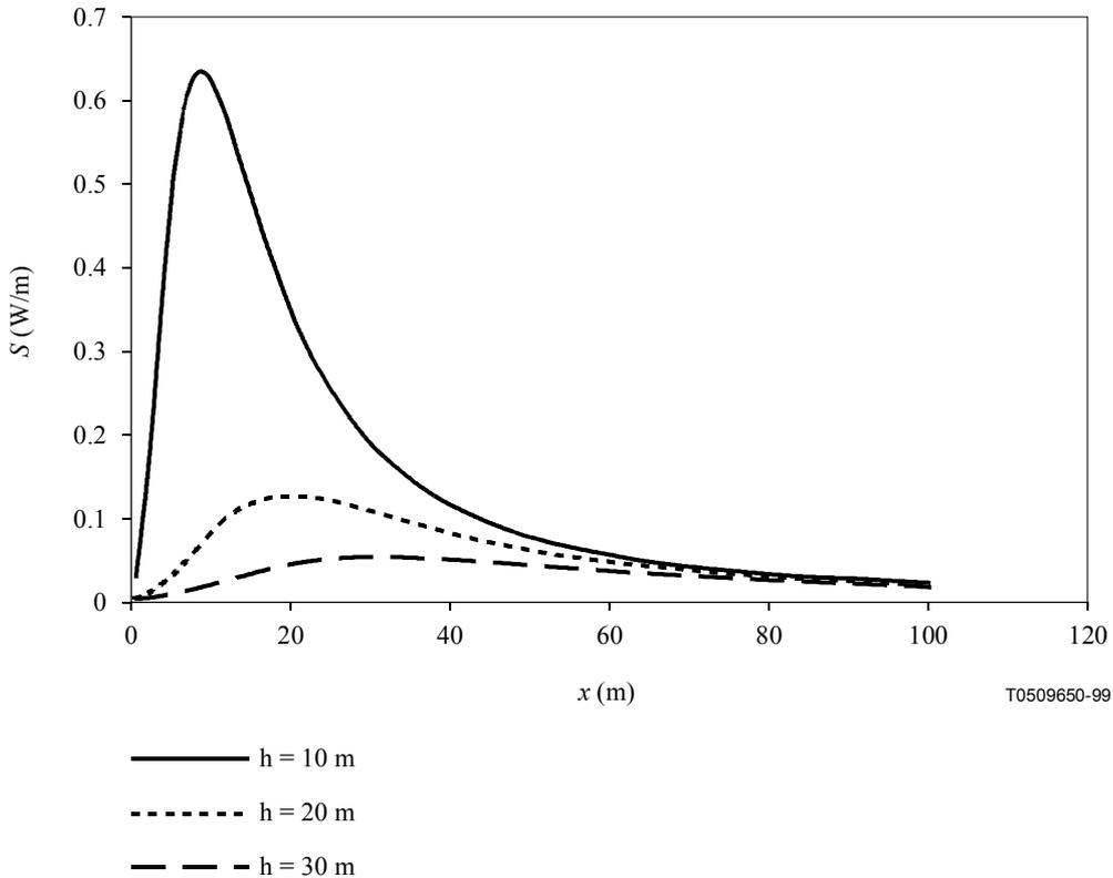
**Figure II.2/K.52 – Power density at the ground level vs. distance from the tower calculated for the example II.1**
