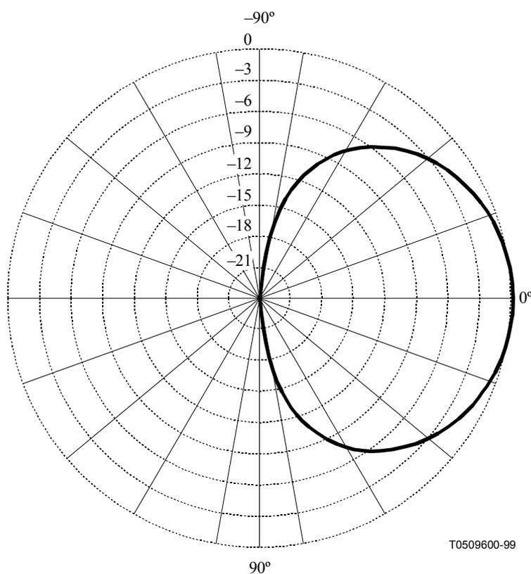
**Figure B.6/K.52 – Vertical pattern for a half-wave dipole**
