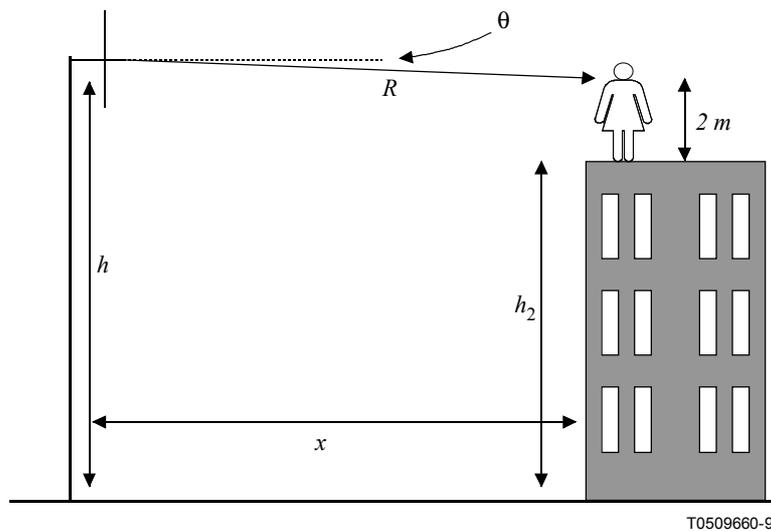
**Figure II.3/K.52 – Sample configuration for calculating exposure at an adjacent building**
