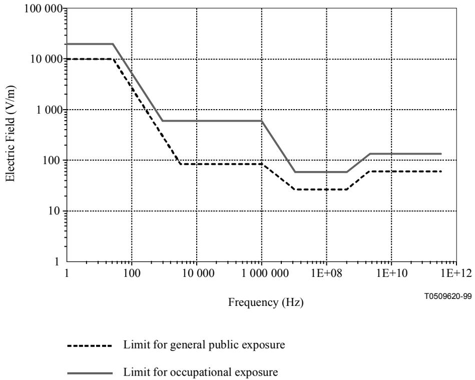
**Figure I.1/K.52 – ICNIRP reference limits for electric field strength**
