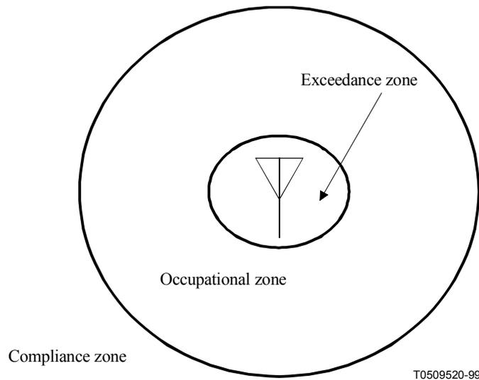
**Figure 1/K.52 – Figurative illustration of exposure zones**
