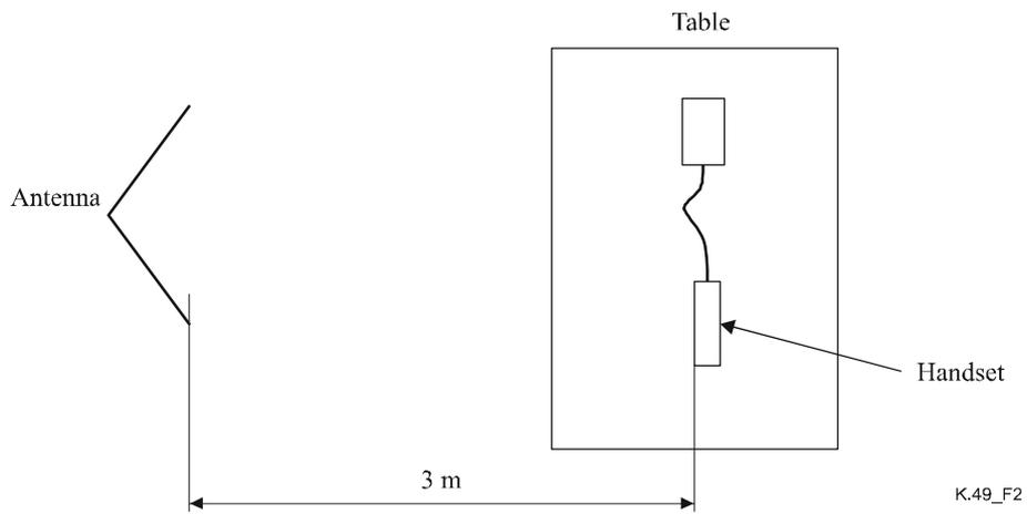
**Figure 2/K.49 – EUT test configuration**
