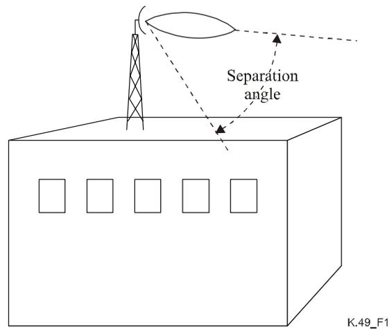
**Figure 1/K.49 – Base station separation angle**
