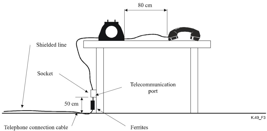
**Figure 3/K.49 – Set-up details of the voice terminal telephone**
