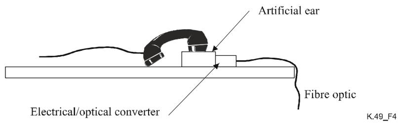
**Figure 4/K.49 – Voice terminal telephone coupled with artificial ear**
