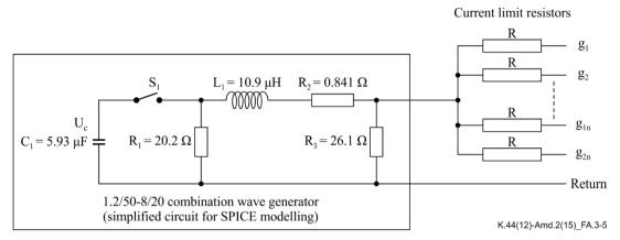
NOTE 1 – The 1.2/50 open-circuit voltage waveshape shall be according to [IEC 60060-1] having a front time of 1.2  $\mu s \pm 30\%$  and a time to half value from virtual zero of 50  $\mu s \pm 20\%$ .
