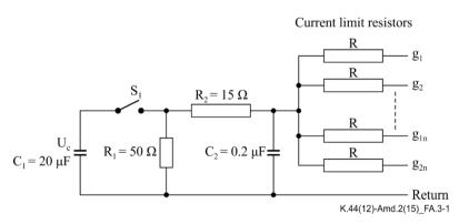
NOTE 1 – The 10/700 open-circuit voltage waveshape shall have a front time of 10  $\mu$ s  $\pm 3~\mu$ s and a time to half value from virtual zero of 700  $\mu$ s  $\pm 144~\mu$ s.
