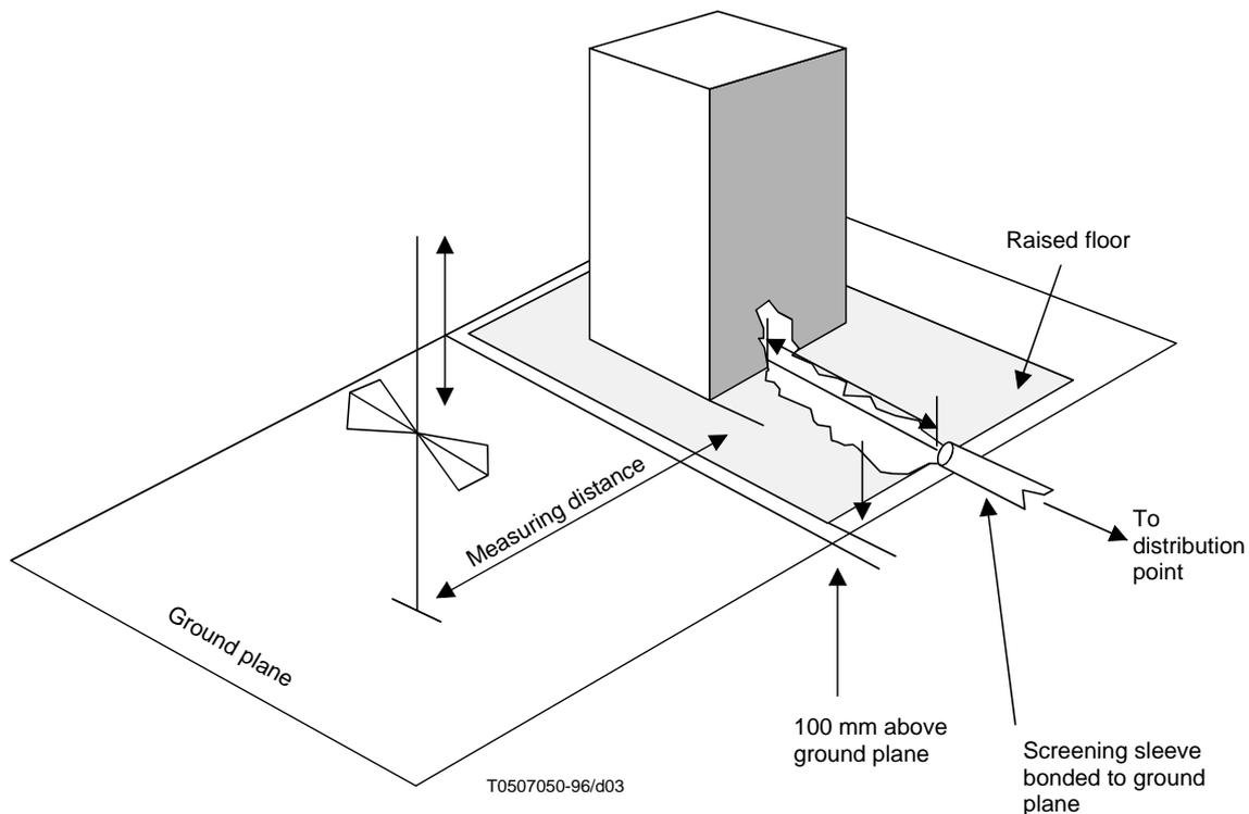
NOTE 1 – If the raised floor does not form part of the screen, the floor panels are removed. The raised floor is isolated from the EUT screen.
