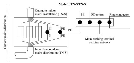
$NOTE-Mode\ 1$  is obligatory if a separation transformer is dedicated to the building and the TN-S system consequently originates at the transformer load side.
