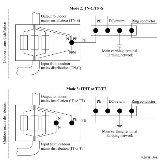
Figure 1 – Arrangements for the transition from the outdoor mains distribution network to the indoor mains
