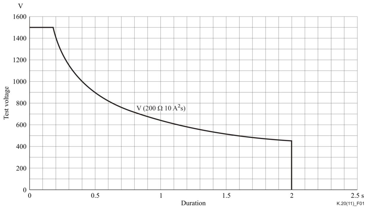
**Figure 1 – Test voltage versus duration to give 10 A<sup>2</sup>s with 200 Ω**
