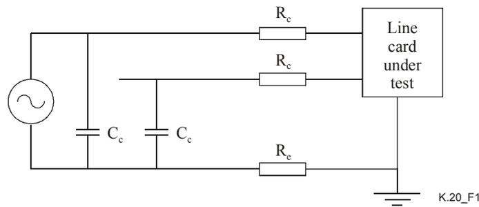
Coupling resistors  $R_c$  represent the line resistances,  $C_c$  represent the line capacitances to earth and  $R_c$  represents the earthing resistance of the overvoltage protectors at the subscriber end of the line.
