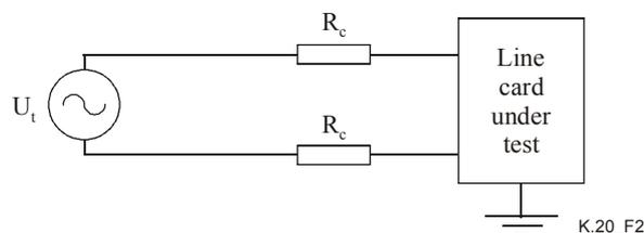
Special test protectors may be used in front of the line card under test if the test is extended to higher voltages.
